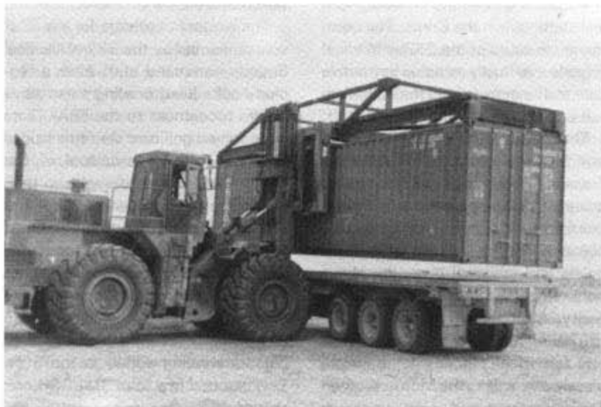
Figure 3. A Rough Terrain Cargo Handler.
