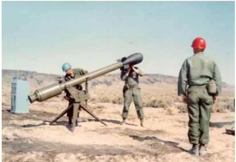
The M28/M29 Davy Crockett Nuclear Weapons System was developed to as a key element of the Pentomic division. Ranges were 2-4 KM Courtesy Army Historical Foundation
