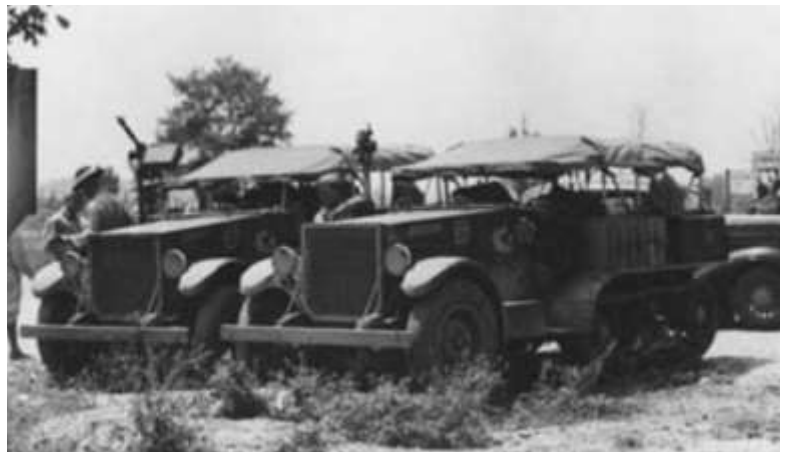
These early half-tracks were unarmored, unlike the M3 half-track that was widely used in WWII.
