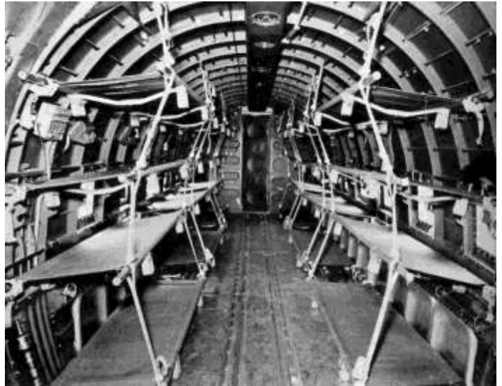
(Above) Interior of a C46 showing the webbing litter straps that were developed to save space. (U.S. Army image)
