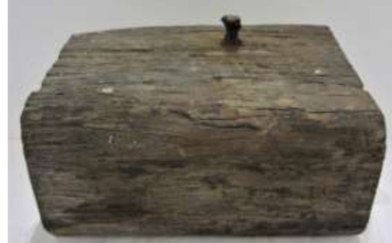
The French used a railroad to assist in the construction of the canal, as did the Americans. (Above) Due to the tropical climate, the railroad ties were made of Lignum Vitae, an especially dense and moisture resistant wood. This piece is only 10" x 5" x 7" but weighs 14 lbs 5 ounces. (Below) A section of the French inverted-U shaped rail. Common in Europe, it was not widely used in the U.S.
