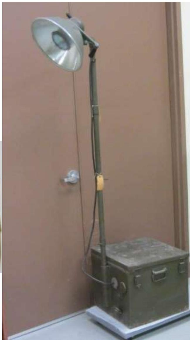
A WWII-manufactured "Field Operating Lamp" that dissembled for travel in its steel base. The lamp was easily set up for operation and could run off various power sources including A/C or D/C current, a portable generator, or from the dry cell batteries stored in the base.
