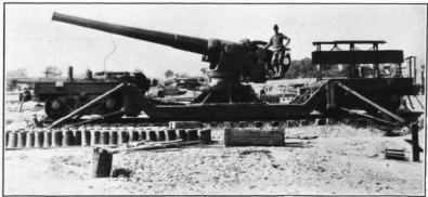
FIG. 11.—United States 7-inch Navy rifle mounted on a pedestal on a railway car. This rifle has a range of about 10 miles and throws a projectile weighing 165 pounds
