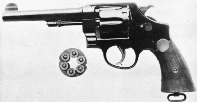
FIG. 67.—Smith & Wesson double-action revolver, model 1917, caliber .45, with adapting clip to take rimless cartridges
