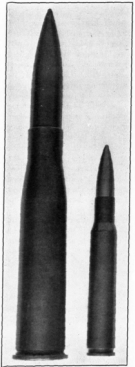
FIG. 71.—German antitank rifle cartridge, compared with the United States Springfield model 1908 cartridge. Full size
