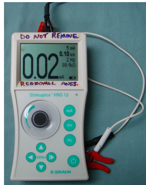
Figure 4-1. HNS 12 nerve stimulator manufactured by B Braun Medical Inc (Bethlehem, Pa)
