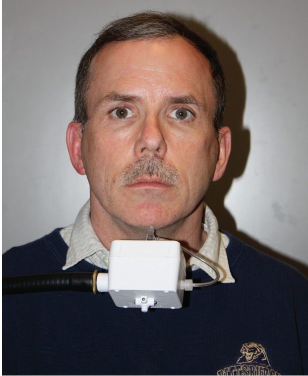
Figure 16-2. A chin joystick controller can be mounted on a boom attached to the chair frame (as shown) or on a plastic yoke placed over the sternum. In addition to driving the power wheelchair, it can be used to operate a tilt-in-space mechanism or environmental control unit.
