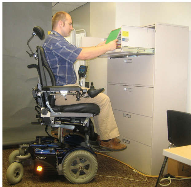
Figure 26-11. A seat elevator can be used to reach higher objects.
