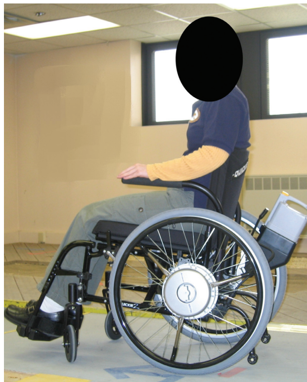
Figure 26-6. A pushrim-activated, power-assist wheelchair.
