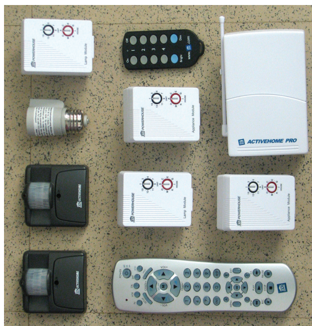
Figure 26-15. The principle components of an electronic aid to daily living.
