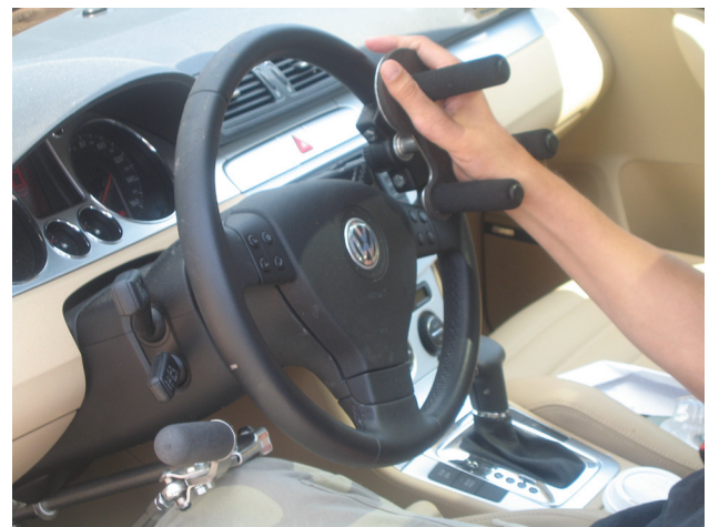
Figure 26-13. A steering knob can aid in driving.
