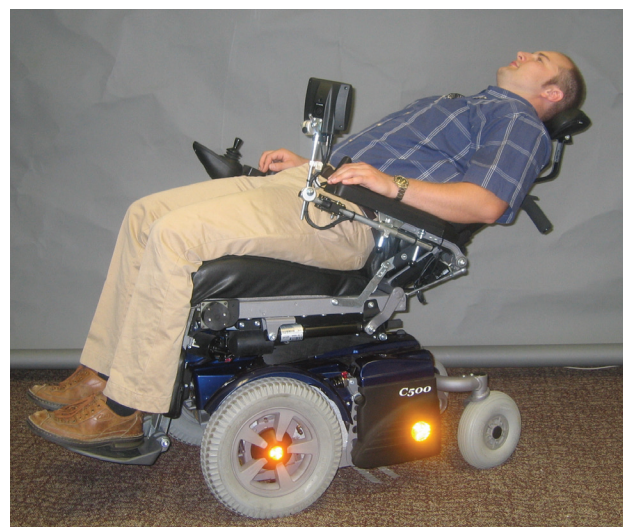
Figure 26-10. A powered reclining backrest system.
