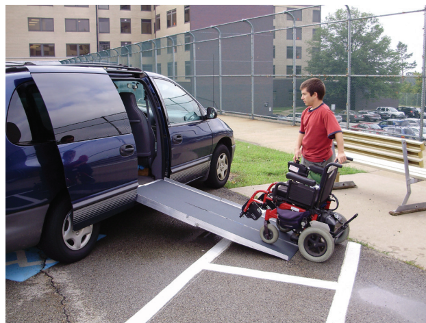
Figure 26-14. A portable wheelchair ramp can be used to access vehicles.
