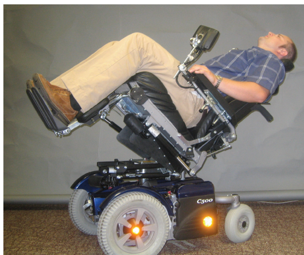
Figure 26-9. A powered tilt seating system.
