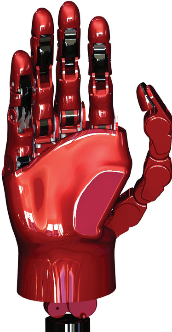
Figure 27-5. Intrinsic hand design, which allows such functions as the pinch-grip, created by the John Hopkins University Applied Physics Laboratory for the Defense Advanced Research Projects Agency (DARPA). All of the actuators are intrinsic within the space of the hand, allowing the device to be fit to patients with a long transradial amputation (actuator technologies such as hydraulics and cobots are excluded due to their large space requirements). 15 brushless DC motors are used to actuate 18 degrees of freedom. Drawing: Courtesy of John Hopkins University Applied Physics Laboratory.
