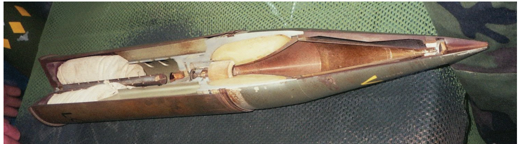
Figure 12. Cross-section image of a high-explosive antitank (HEAT) round. Note the reverse cone of metal liner in the mid-section and the exploding charge at the base of the round. Image courtesy of Wikimedia Commons.
