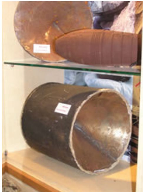
Figure 13. (Left) An explosively formed projectile is an IED variant consisting of a cylindrical casing, closed with a concave-shaped metal plate facing inward, and an internal explosive charge. On detonation, the concave plate is propelled out of the casing and can inflict catastrophic injury. Image courtesy of Defense-Update.com.
