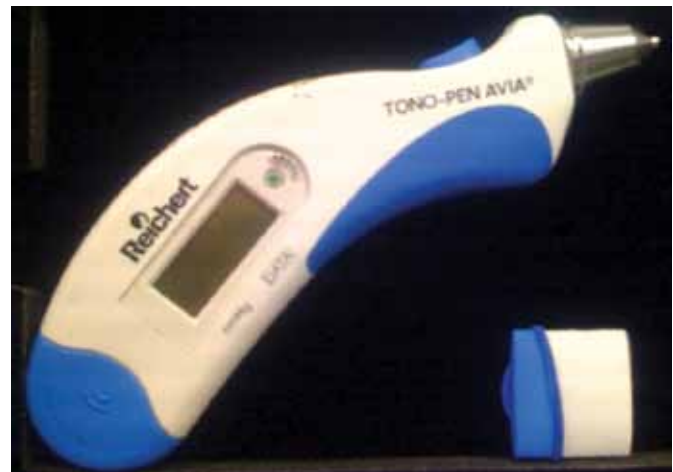
Figure 12. The Tono-Pen® is a portable device that can be used by ophthalmic and nonophthalmic personnel to accurately measure intraocular pressure.
