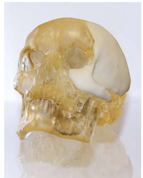
(Left) A computer model of a skull based on CT scan data. (Right) An acrylic skull created on a rapid prototyping machine based on computer data similar to that shown above and on the left. Source: 3D Medical Applications Center
