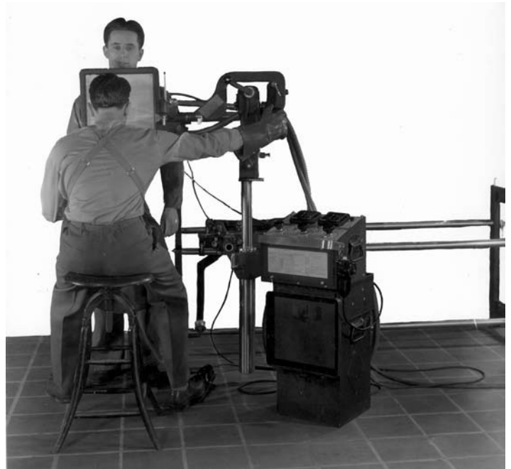
▲ (Left and Right) Demonstrations of a portable X-ray apparatus as used in the field, Army Medical School, 1941. Source: Walter Reed Army Medical Center History Office, PAO Historical Collection
