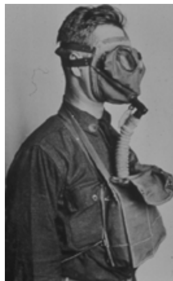
Fig. 3-8. The British small-box respirator, introduced in 1916 and seen in 1918 in this photograph, was vastly more satisfactory than the earlier British helmets. The wearer breathed through a mouthpiece (like that worn by a scuba diver). Since a spring clip was applied to the nose, only air that had passed through the mouthpiece could enter the lungs. An absolute seal between the face and mask was unnecessary. The mouthpiece was connected by a tube to the canister containing neutralizing chemicals, which was worn around the trunk. Although the small-box respirator was much more protective than its predecessors, it was probably even less user-friendly. Photograph: Courtesy of Pictorial History, Gas Defense Division, Chemical Warfare Service, Vol 5, Edgewood Historical Files. Held at Chemical and Biological Defense Command Historical Research and Response Team, Aberdeen Proving Ground, Md.
