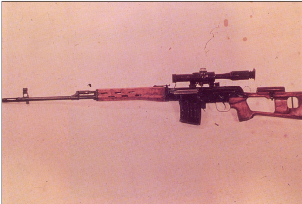
Fig. 1-14. The 7.62-mm Snayperskaya Vintovka Dragunova (SVD) is a semiautomatic gas-operated rifle that fires the 7.62 x 54R round shown in Figure 1-3. Its telescopic sights make it an excellent sniper's weapon.
