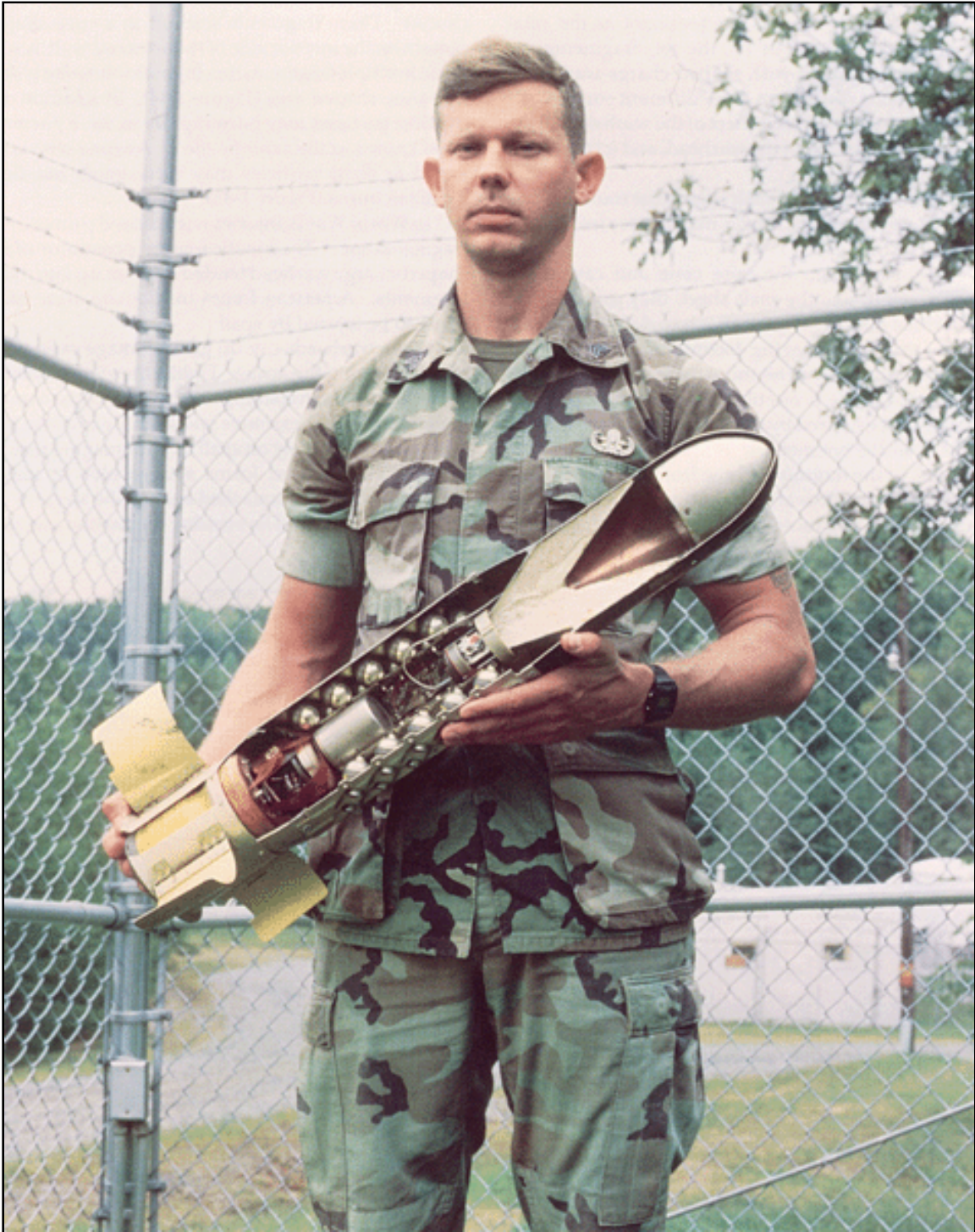
Fig. 1-39. The marine holds a cutaway version of a Dragon medium antitank missile, in which the characteristic hollow shape can be clearly seen.
