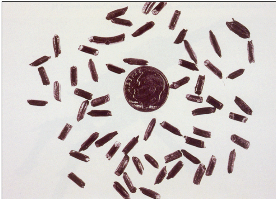
Fig. 1-60. Some of the fragments that are formed from the notched wire in the VOG-17 round after it has been detonated are compared in size to a dime.
