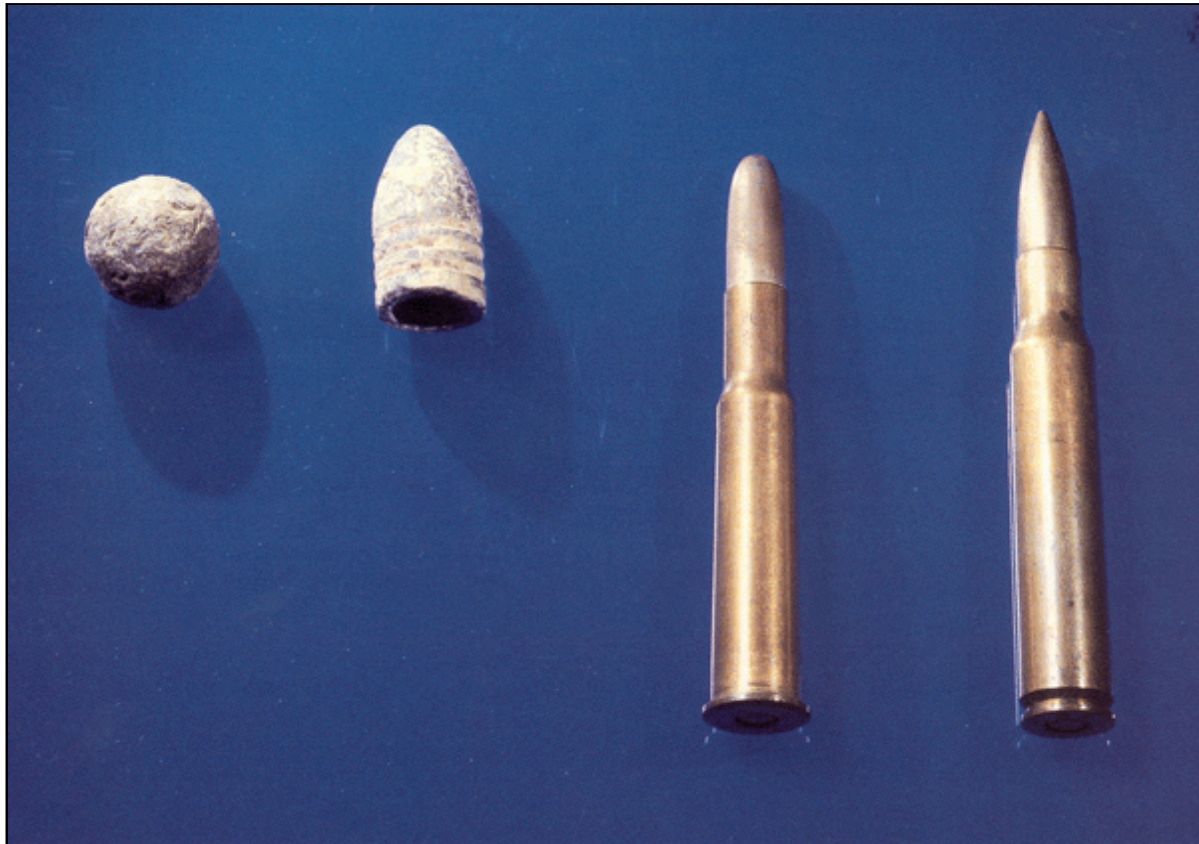
Fig. 3-1. Some bullets of historical importance are, from left to right: musket ball, 69-caliber smooth bore, dating from about 1840; Minie bullet, 55-caliber, dating from about 1555; blunt-nose, 30–40 Krag-Jorgensen, dating from about 1892; spitzer, 1903 Springfield, dating from about 1906.
