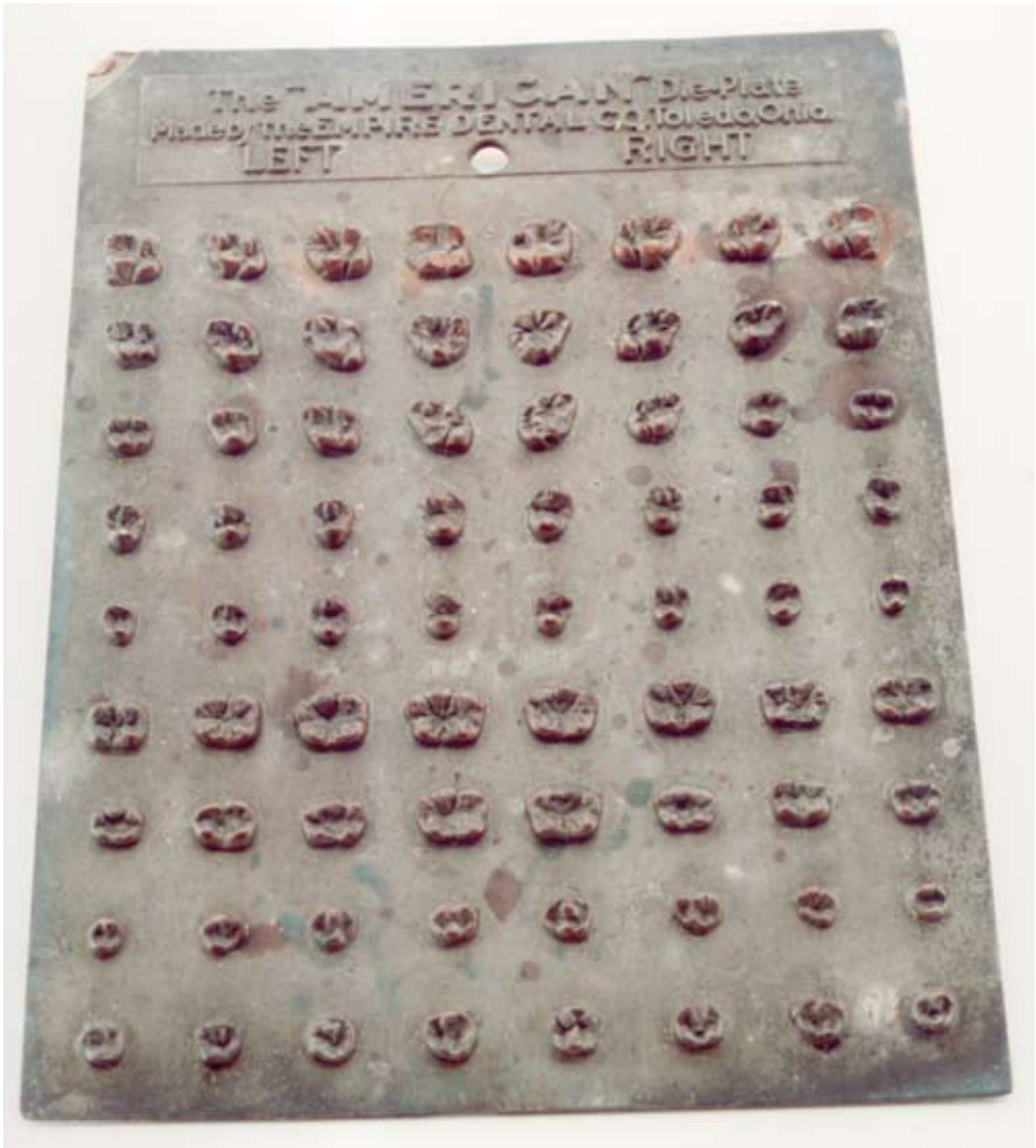
Die plate, circa 1875. This die plate was used to swage (pound into shape) the occlusal surface of a shell crown made of 22K plate gold. By 1955 this technique was superseded by cast gold crowns.
