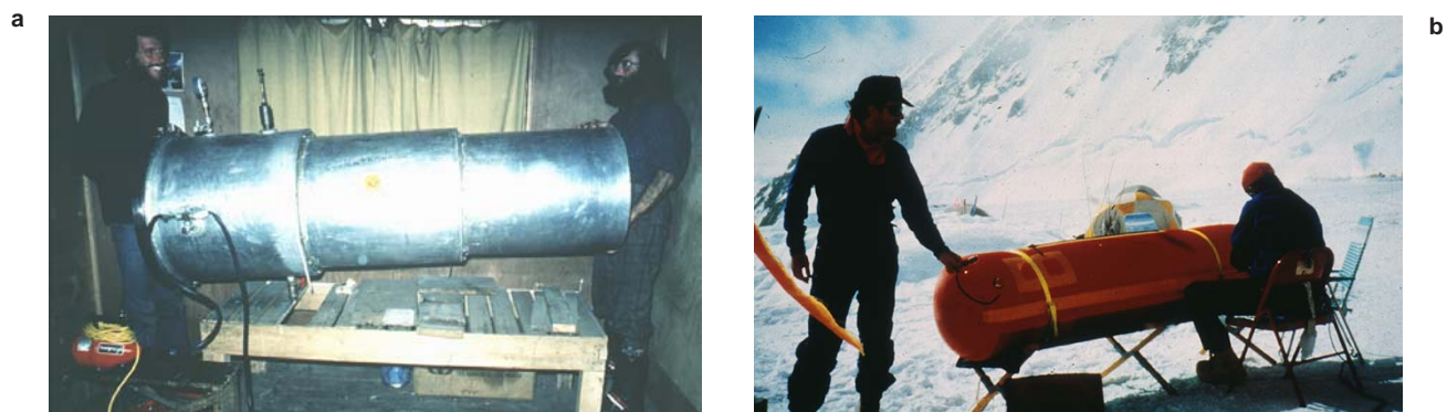
Fig. 24-9. Increasing pressure by descent or by putting a patient in a hyperbaric chamber effectively treats acute mountain sickness (AMS) and high-altitude cerebral edema (HACE). Hyperbaric pressurization, descent, and oxygen therapy are of equivalent effectiveness for treating AMS and HACE. (a) This pressure chamber was first used in Pheriche, Nepal, in 1975 for recompression of patients ill with AMS or HACE. (b) A fabric hyperbaric chamber has the advantage over portable oxygen cylinders of being lightweight, being easy to transport, and offering simulated descent for as long as the operator can pressurize the chamber by manual pump.
