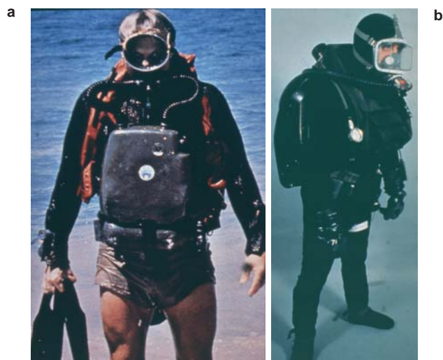
Fig. 37-11. (a) A US Navy SEAL ( sea, air, land ) diver is wearing the Draeger LAR V underwater breathing apparatus (UBA). (b) A SEAL diver is dressed in an Mk 16 UBA. Photograph: Courtesy of US Special Operations Command, MacDill Air Force Base, Tampa, Fla.
