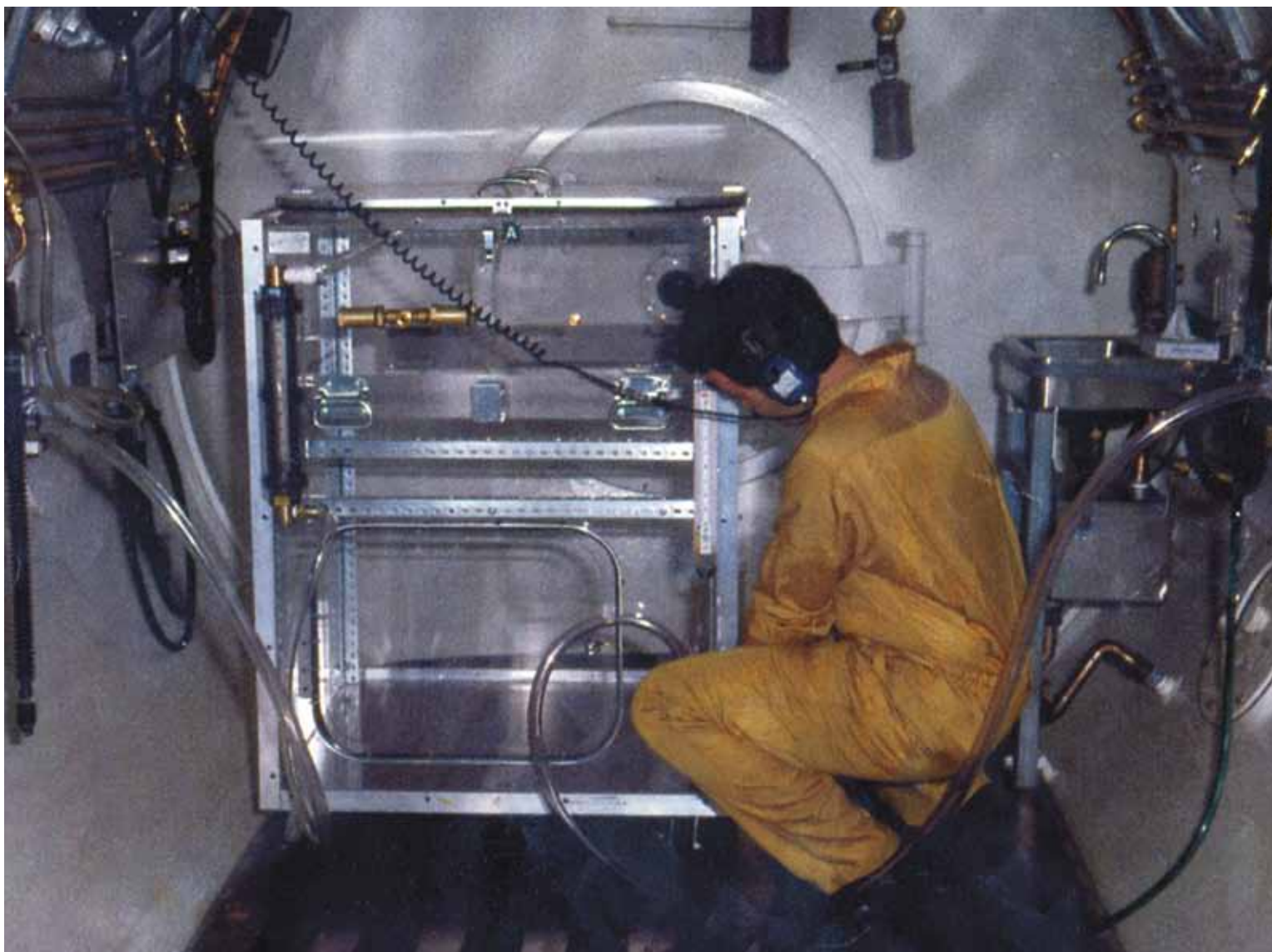
Air Force Staff Sergeant Dave Nelson prepares an animal isolation box for a simulated hypobaric dive in the early 1990s designed to test the effects of pressure and oxygen on the physiology of tissue repair. The animal isolation boxes, which were specially constructed for use at depth, permitted investigators to accompany animal models inside the chamber during testing without being exposed to the same breathing environment. (NCP 17351)
