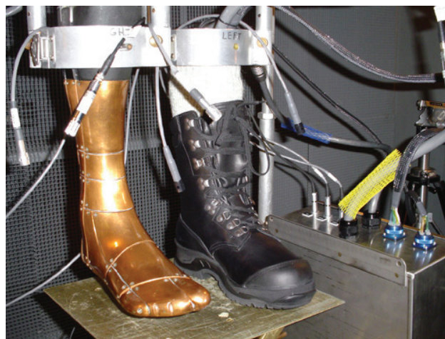
Fig. 1-7. Biophysical testing models, such as the copper foot, have been highly refined by the US Army for thermal insulating and vapor transmissibility properties of individual clothing. This copper foot at the USARIEM laboratory is being used to test a Norwegian boot. Photograph: Courtesy of USARIEM, T Rice, Public Affairs Office.
