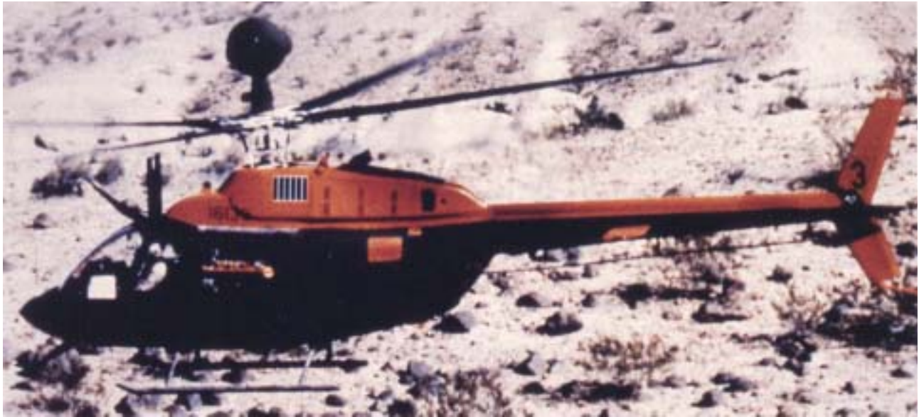
Fig. 1-9. The OH-58D Advanced Scout Helicopter was designed for enhanced aerial reconnaissance; intelligence gathering; and target detection, acquisition, and designation. It serves as an excellent example of the many different, potentially adverse exposures that may be inherent in new materiel. Under the Health Hazard Assessment Program, the OH-58D was evaluated for the following potential hazards to human health: lasers contained in the ball on top of the main rotor; heat stress resulting from the large number of electronic items carried in board; engine-exhaust products that could enter the cockpit; whole-body vibration; and the crash worthiness of the seats, which had been used on other aircraft and were reported to have been associated with excessive spinal injuries during crash landings. Source: Rowden SE, McIntosh RM. The health hazard assessment program: Occupational health for the soldier in the field. Medical Bulletin of the US Army Medical Department . 1988;2:7–13. PB 8-88. Photograph: USAEHA file.
