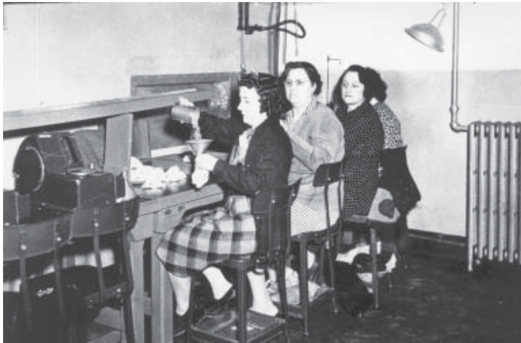
Fig. 1-3. This April 1942 photograph from the U.S. Army Ordnance Department shows workers measuring smokeless powder, which contains a nitrate or nitroglycerin compound, and pouring the powder into bags, which will later be used to propel projectiles from guns or cannons. Although the dangers of skin absorption in the munitions industry and the need for washable work clothing were recognized in the World War I era, these early–World War II workers labored in street clothes without any evidence of concern about skin contact with the powder. Source: Hamilton A. Exploring the Dangerous Trades, the Autobiography of Alice Hamilton, M.D. Boston: Little, Brown and Co; 1943. Photograph: U.S. Army Ordnance Department, 1942.
