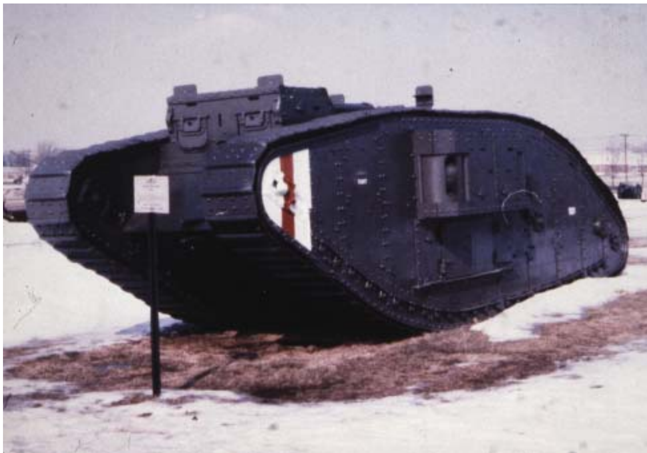
Fig.1-5. The first major tank battle, the Battle of Cambrai, took place on 20 November 1917 in northern France. From behind the British front, 378 ironclads (an early name for tanks) similar to the British Mark IV shown above moved toward the Hindenburg Line. The Mark IV had five .303-caliber Lewis machine guns and armor only thick enough to protect against small-arms fire. The inside of the tank was one large compartment in which the crew were exposed to combustion products from the weapons and exhaust from the petrol engine. Sources: (1) Gaydos JC. A historical view of occupational health for the soldier. Medical Bulletin of the US Army Medical Department . 1988;2:4–6. PB 8-88.(2) Cooper B. The Ironclads of Cambrai . London: Souvenir Press; 1967. Photograph: Courtesy of Colonel Joel C. Gaydos, Bethesda, Md.
