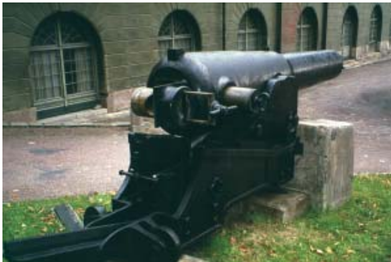
Fig. 10-3. An innovation that significantly increased the possibility that soldiers would be exposed to propellant combustion products was the rear- or breech-loaded cannon. The breech-loaded cannon was conceived at least as early as the Middle Ages but manufacturers could not produce a tight seal that would prevent leakage of propulsion pressure. A simple mechanism that was found to be effective was the “sliding breech block,” which was used in this 19th-century Swedish cannon. After the breech door was closed, the piston on the right (the breech block) was moved to the left to complete the breech seal. Another 19th-century innovation was the brass cartridge case, which was forced tightly against the inside of the barrel. Other devices used to seal the breech include the interrupted screw breech block (sections of thread are cut away, allowing the breech block to be locked with only a turn of a few degrees) and the soft obturator ring. The obturator ring, located directly in front of the interrupted screw breech block, is forced against the breech block by the propellant explosion, forming a tight seal. Sources: (1) Holmquist BM, Gripstad B. Swedish Weaponry Since 1630 . The Defence Matériel Administration of Sweden. The Royal Army Museum. Arlöv, Sweden: Berlings; 1982: 66. (2) Harding D, ed. Weapons: An International Encyclopedia from 5000 BC to AD 2000 . Leicester, England: Galley Press (WH Smith and Son Limited); 1984.
