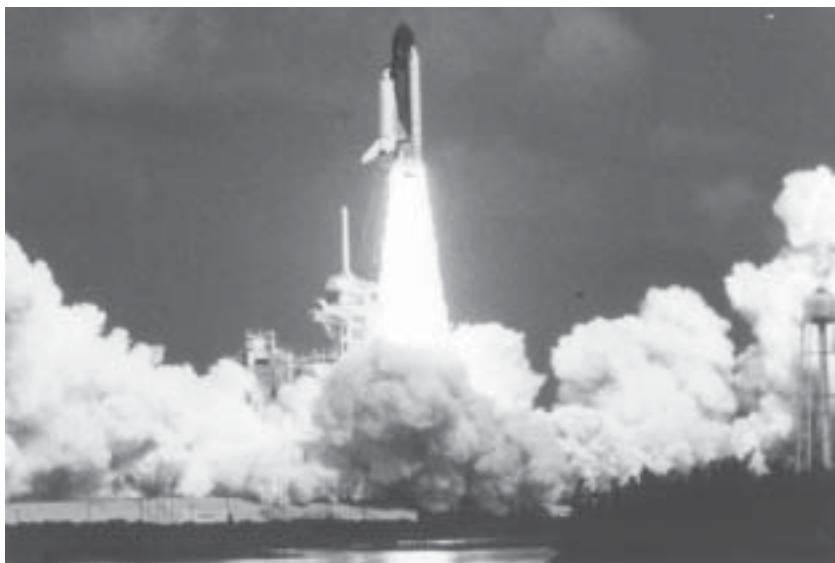
Fig. 10-9. The space shuttle Atlantis is shown being launched from the Kennedy Space Center, Florida, at 9:56 a.m. (EDT) on 31 July 1992. The large quantity of white smoke surrounding Launch Complex 39 is hydrogen chloride that was produced during combustion of the shuttle's perchlorate-based, solid rocket propellant. Photograph: Courtesy of National Aeronautics and Space Administration, Houston, Tex. 31 July 1991. Photograph STS046-(S)-082.
