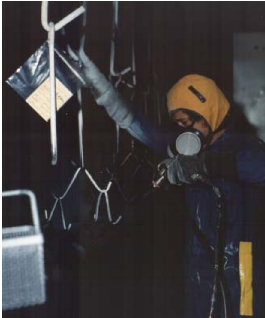
Fig. 12-3. Worker performs spray painting on drag-line component parts against a waterfall paint booth. During such operations, workers are at risk of inhaling aerosolized lead unless protective respirators are worn properly. Source: US Army, Anniston Army Depot, Anniston, Ala.
