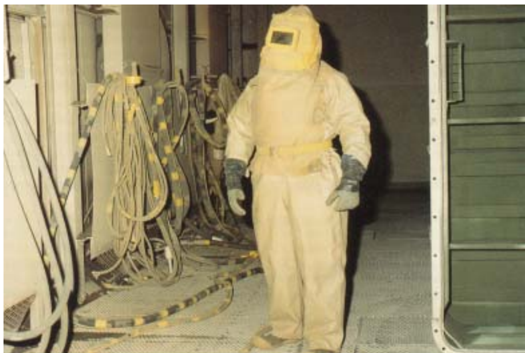
Fig. 12-12. Cumbersome protective gear (including a respirator, hooded chemical-resistant suit, gloves, and boots), worn for prolonged periods of time in sandblasting operations, imposes both physiological and psychological demands on the worker. Excessive physiological demands often manifest as heat stress. The inability to tolerate the psychological demands may manifest as anxiety or claustrophobia. Source: US Army, Anniston Army Depot, Anniston, Ala.
