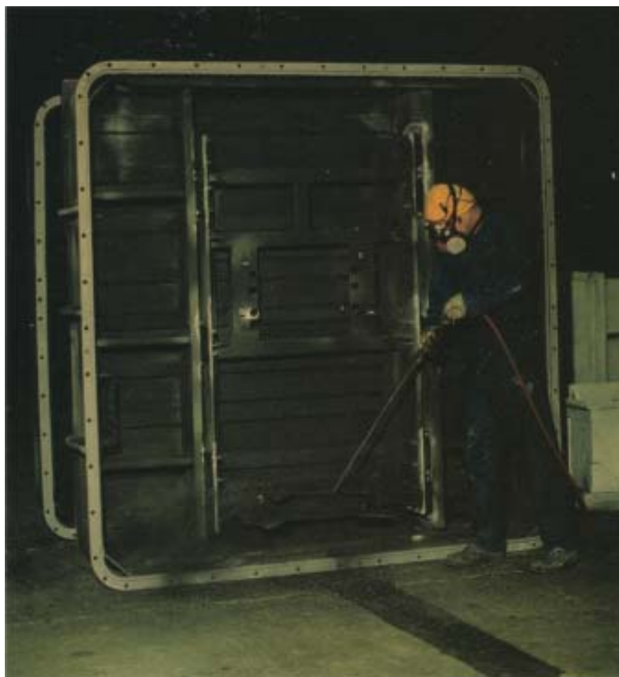
Fig. 12-4. A worker uses compressed air in the painting preparation process. This process is often called “blasting” or “sandblasting” if sand is the abrasive material. Exposure to lead can result from the dust from the residual paint. Source: US Army, Anniston Army Depot, Anniston, Ala.
