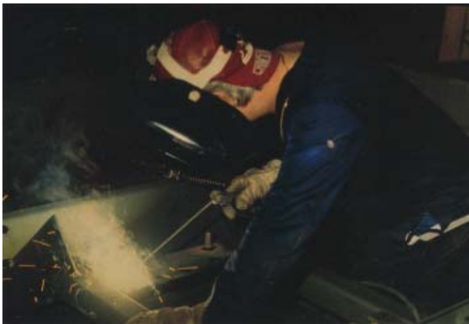
Fig. 12-6. Welding on lead-coated materials places the worker at risk of lead intoxication. Here, exposure may result from the vaporization of lead in paint that was incompletely removed from the surface before the welding was begun. Source: US Army, Anniston Army Depot, Anniston, Ala.
