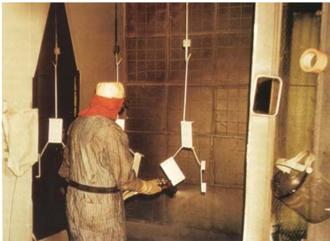
Fig. 13-3. The operator in this walk-in spray booth is wearing coveralls, gloves, a head cover, and an air-purifying respirator. He has also positioned the items to be painted between himself and the booth's exhaust ventilation. This serves two purposes: it minimizes the potential for the painter's exposure and it prevents vapors and aerosols from leaving the spray booth.
