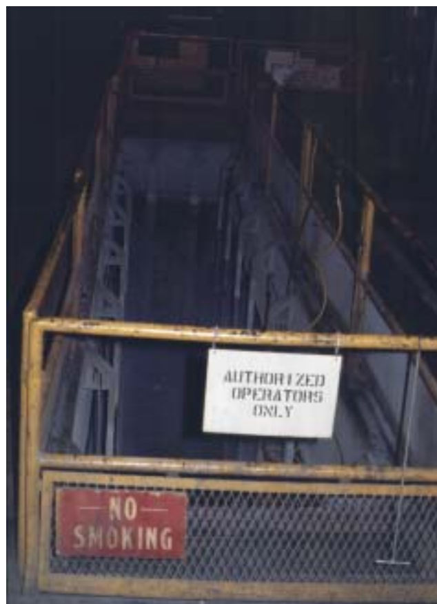
Fig. 13-1. A typical degreasing tank. Vapor degreasing is accomplished by lowering the object to be cleaned into the vapor zone above the liquid solvent. Solvent vapors condense on the cold item and loosen grease and oil, which then collect in the bottom of the tank. Condensing coils located near the top of the tank condense the solvent vapors, which collect in the condensate trough and are returned to the reservoir. The item is held in the vapor zone until the parts reach the temperature of the solvent vapor. At that time, condensation stops and the item is dry.
