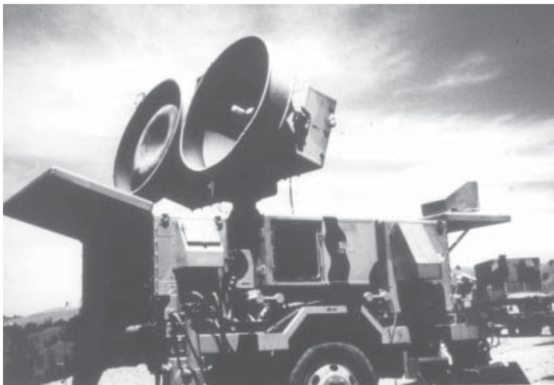
Fig. 15-11. The high-power illuminator radar (HIPIR) is an acquisition radar of the Hawk air-defense system.
