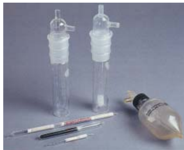
Fig. 4-12. The midget impinger shown in the left background is used to collect contaminants in a liquid medium; the midget fritted impinger shown on the right background breaks up contaminated gases into tiny bubbles, thereby increasing the collection efficiency. The impinger shown in the right foreground is designed to collect samples but not leak into the pump. Collection tubes containing Firebrick, activated charcoal, and silica gel, center foreground, top to bottom, are used to collect various gases and vapors for laboratory analysis.
