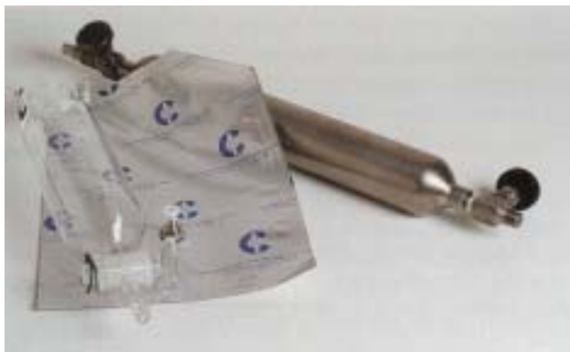
Fig. 4-14. Stainless steel, right, or glass, left, evacuation containers have valves to control the collection of grab samples of worksite air into rigid containers of known volume. The flexible collection bags, center, usually have fittings that connect to air pumps, which fill the bag with the air sample.
