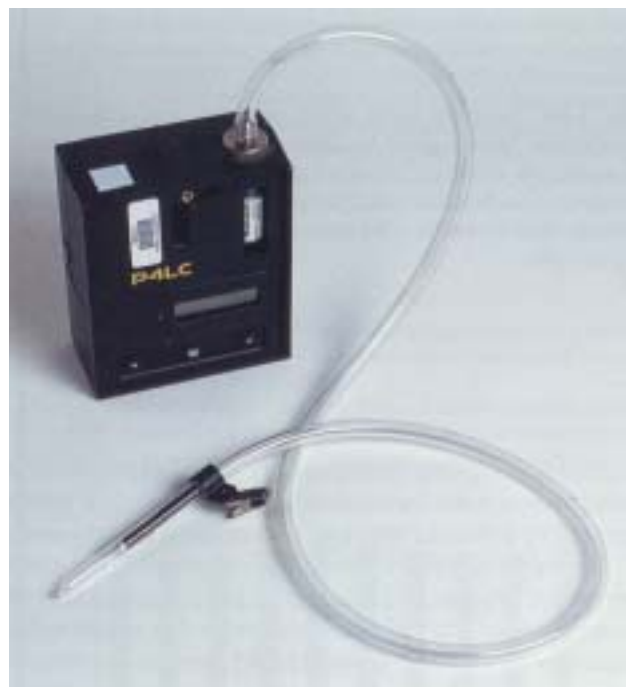
Fig. 4-11. This DuPont P4LC constant flow pump with its sampling tube attached is a sampling train used to collect many kinds of gas and vapor contaminants. A particulate sampling train would have a filter or filter/cyclone collection device. Constant flow pumps use microprocessors to sense airflow and alter pump speed to maintain a known collection rate.
