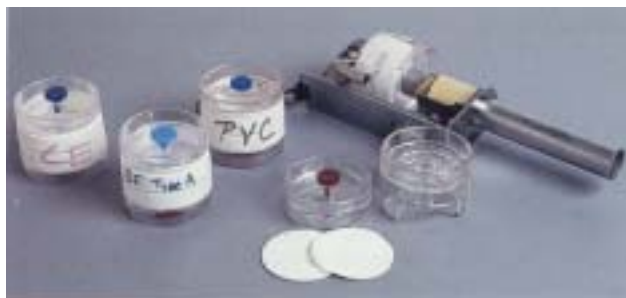
Fig. 4-10. Particulate filters, left to right: cellulose ester; glass fiber; polyvinyl chloride; a filter taken apart to show the body, support pad, and filter disk; and a filter mounted in a cyclone device that is used to separate out the respirable aerosols. These particulate collection filter assemblies differ according to the laboratory requirements for extracting the hazardous material collected from the filter media.
