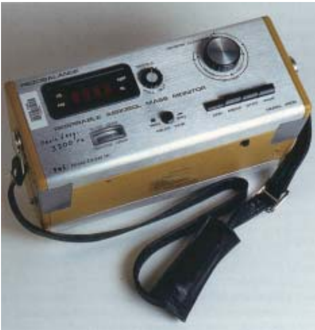
Fig. 4-8. This TSI Respirable Aerosol Mass Monitor Model 3500 uses the frequency changes of piezo crystals to determine the mass of 0.01–10 \mu particles in air.
