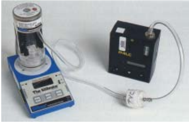
Fig. 4-15. The Gilian Instrument Corporation's Gilibrator Bubble Generator provides an efficient method of determining airflow rates before, during, and after sample collection.
