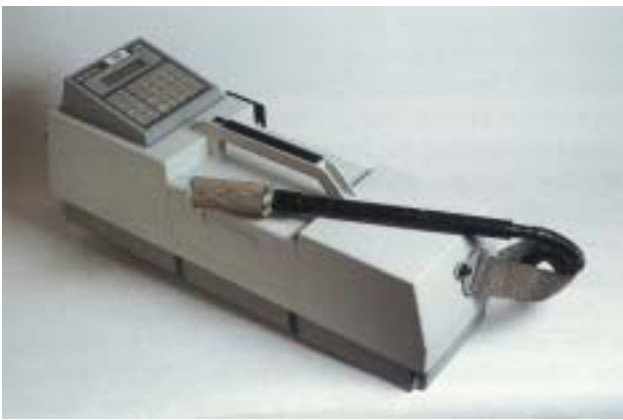
Fig. 4-7. This MIRAN 1B2 infrared gas analyzer provides sub-ppm measurement of a wide variety of gases and vapors. This instrument or a variant is frequently used to monitor for ethylene oxide and waste anesthetics in army medical treatment facilities.
