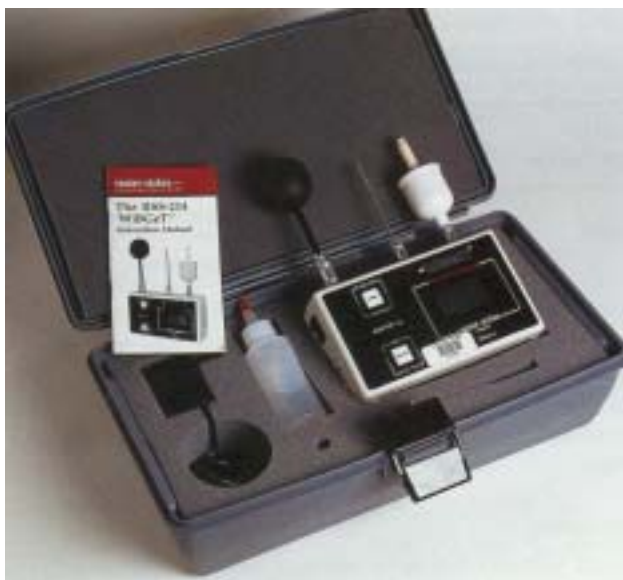
Fig. 4-4. This Reuter Stokes RSS-214 WiBGt Wet Bulb Globe Thermometer electronically records the wet bulb, dry bulb, and black globe temperatures, then calculates a heat-stress index that is used to determine the protection necessary for the stresses of excessive heat. Heat stress is the subject of US Army Research Institute of Environmental Medicine (USARIEM) Technical Note 91-1, Sustaining Health and Performance in the Desert , 15 which can be consulted for further information.
