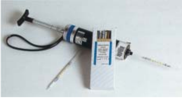
Fig. 4-6. This GASTEC/Sensidyne pump, model 800 with formaldehyde low range (0.1–5 ppm) detector tubes, is used to rapidly screen areas for formaldehyde gas. Other types of tubes are available to screen for many common chemicals. Each carton contains specific instructions for sample volumes.
