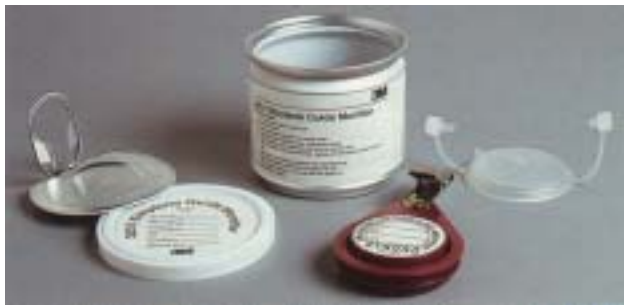
Fig. 4-13. This 3M Gas Badge, shown in front of its shipping container, is used to monitor for exposure to ethylene oxide; air pumps or other sampling-train components are unnecessary.
