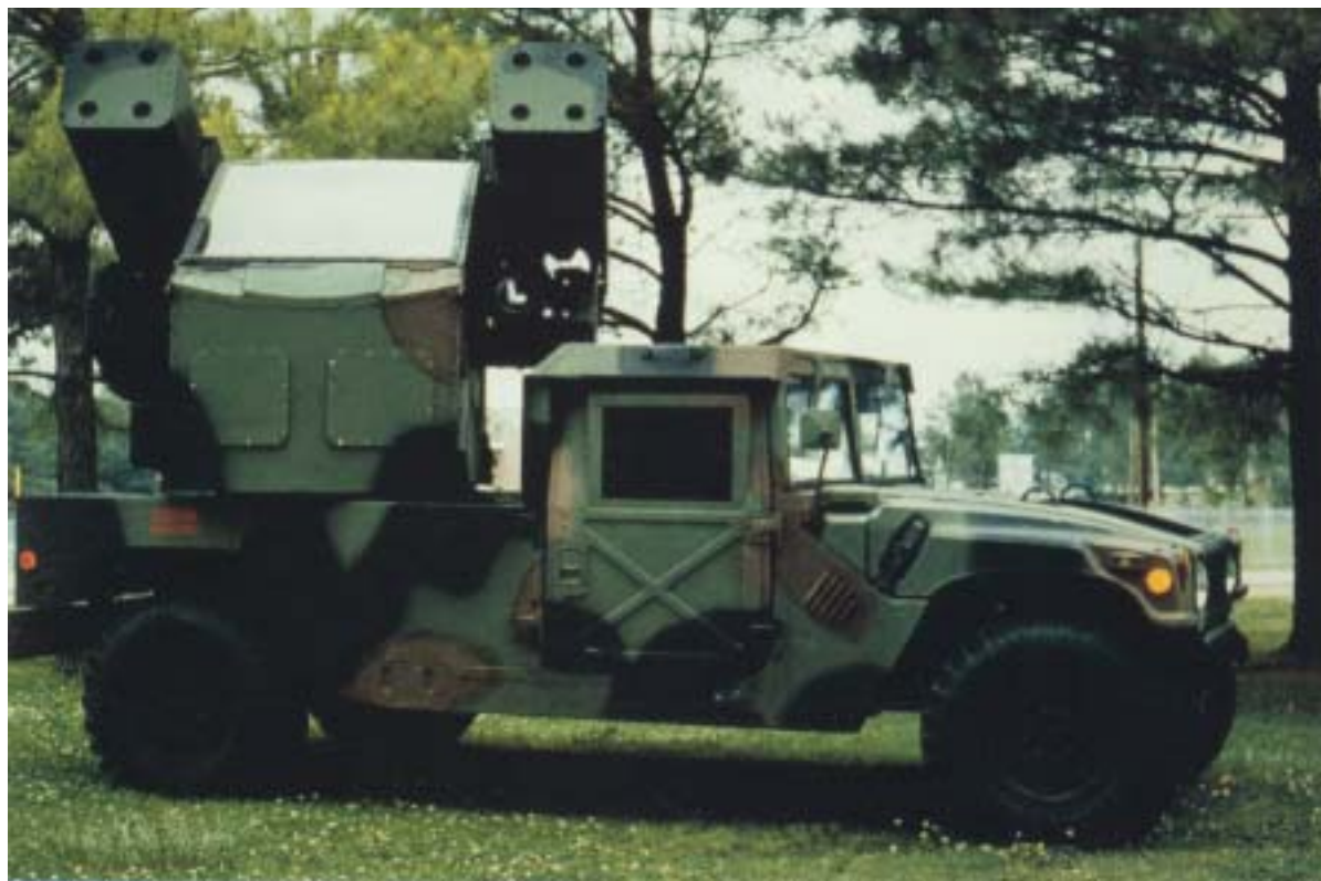
Fig. 6-10. Avenger Air Defense System. The Avenger enhances the Stinger missile with new capabilities such as shoot on the move, day/night operations, and multiple rapid sequential engagements. Avenger integrates the Stinger missile, a gyrostabilized turret, forward-looking infrared, laser rangefinder, identification of friend or foe, and a .50-caliber machine gun. It is operated either from the vehicle cab or remotely by a crew of two: the driver and the gunner.
