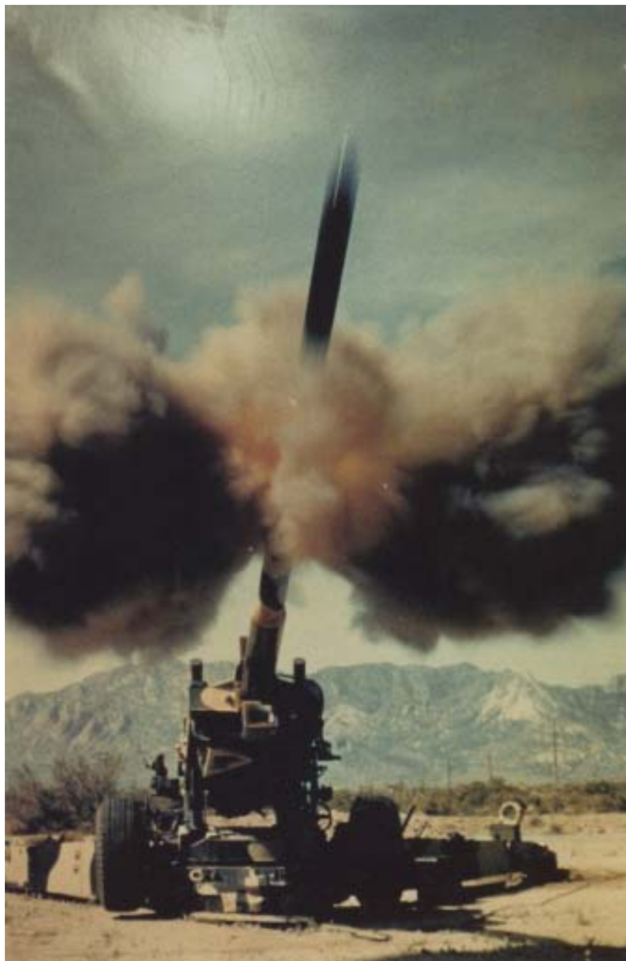
Fig. 6-1. The M198 155-mm Towed Howitzer. The M198 is a helicopter-transportable 155-mm medium towed howitzer. It has a conventional split-trail carriage and uses a hydropneumatic recoil mechanism. The maximum rate of fire is 4 rounds per minute for the first 3 minutes and 2 rounds per minute sustained. It is capable of firing a 96-pound rocket-assisted projectile to a range of 30 km.
