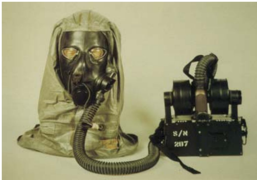
Fig. 6-12. M43A1 Aircraft Chemical-Biological (CB) Mask. The M43A1 mask consists of a form-fitting facepiece with spherical lenses fitted close to the eyes, an integrally attached CB hood and skull-type suspension system (fitted over and suspended from the head), an inhalation-air distribution assembly for regulating air flow to the mouth and nose, lenses and hood assembly, an exhalation valve assembly, an electronic microphone, and a portable motor-blower filter assembly for maintaining overpressure in the mask and hood.
