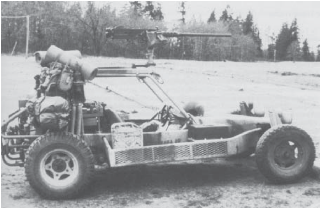
Fig. 6-19. Fast Attack Vehicle (FAV). The FAV is similar to a dune buggy and is used by the U.S. Army’s Special Forces units. Although it has limited cargo-carrying and fuel capacity, it was used during Operation Desert Storm and reportedly carried the first coalition forces into Kuwait City.
