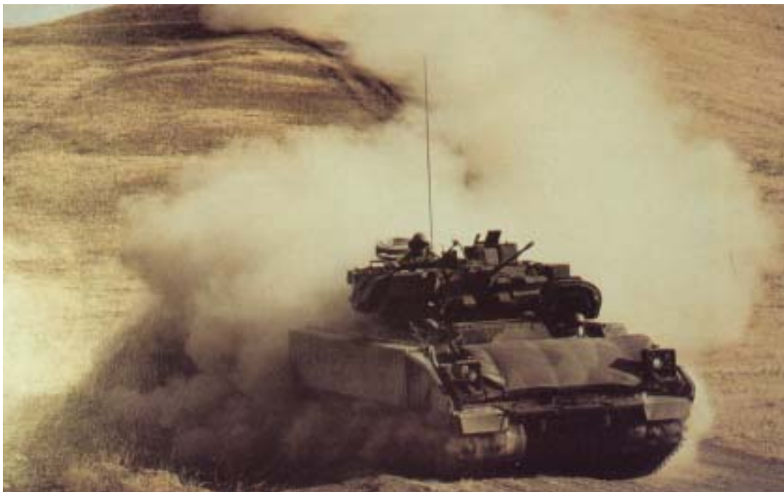
Fig. 6-3. The Bradley Fighting Vehicle (BFV). The BFV is named for the late General of the Army Omar N. Bradley. Two versions, the M2 Infantry Fighting Vehicle (IFV) and the M3 Cavalry Fighting Vehicle (CFV), are externally indistinguishable and have the same armament and automotive performance. The major difference between the M2 and M3 is the arrangement of the crew compartment and internal storage. The armament includes the M242 25-mm chain gun, M240 7.62-mm coaxial machine gun, and a TOW (tube-launched, optically-tracked, wire-guided) antitank missile launcher.
