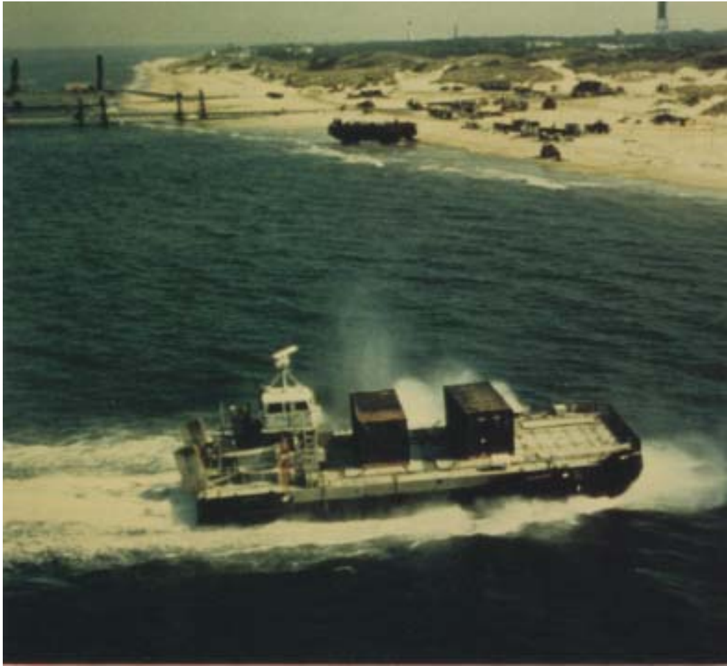
Fig. 6-6. The Lighter, Air Cushion Vehicle, 30-Ton Capacity (LACV-30). The LACV-30 is capable of around-the-clock operations regardless of the weather. It easily transports wheeled and tracked vehicles, containers, and bulk cargo on its 1,660 ft 2 deck. Its maximum payload is 35 tons, cruise speed is 45 mph, and endurance is 8 to 10 hours. U.S. Army transportation units received their first production craft in 1982.
