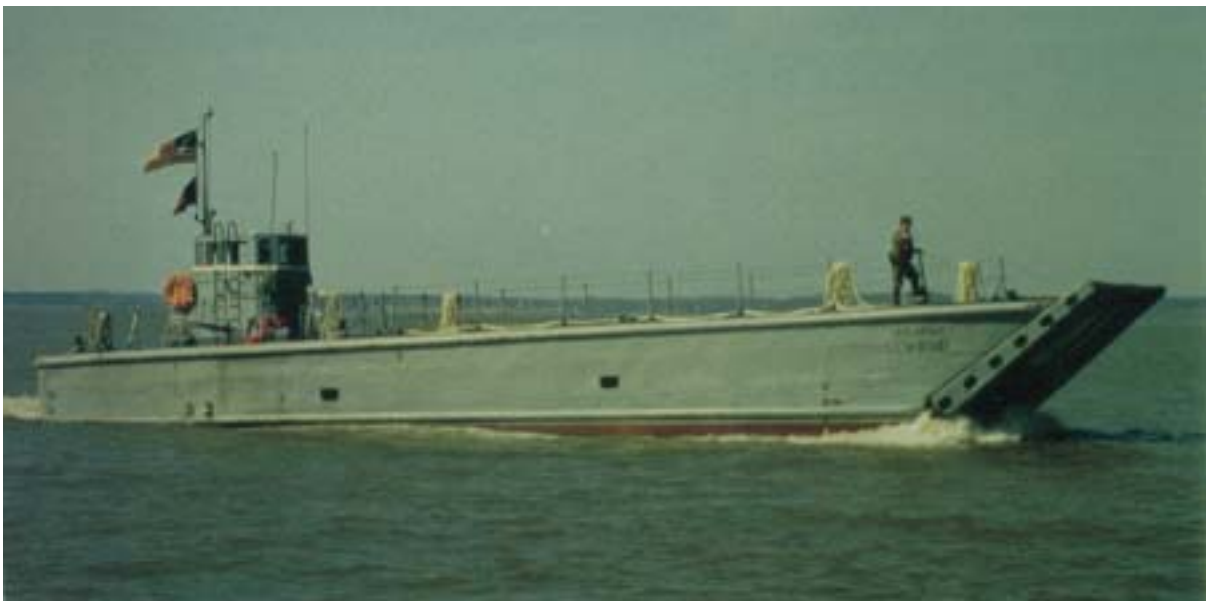
Fig. 6-17. Landing Craft Mechanized-8 (LCM-8) Mod 1, Service Life Extension Program (SLEP). The LCM-8, Mod 1, SLEP is a product-improvement program intended to restore the mission capability and supportability characteristics of the existing fleet and extend its service life by 20 years. The primary modification is the replacement of the old twin Detroit Diesel 6-71 engines with new 12V-71 diesel engines and associated hardware. The army has a fleet of approximately 96 of these vessels assigned to Transportation Medium Boat Companies.
