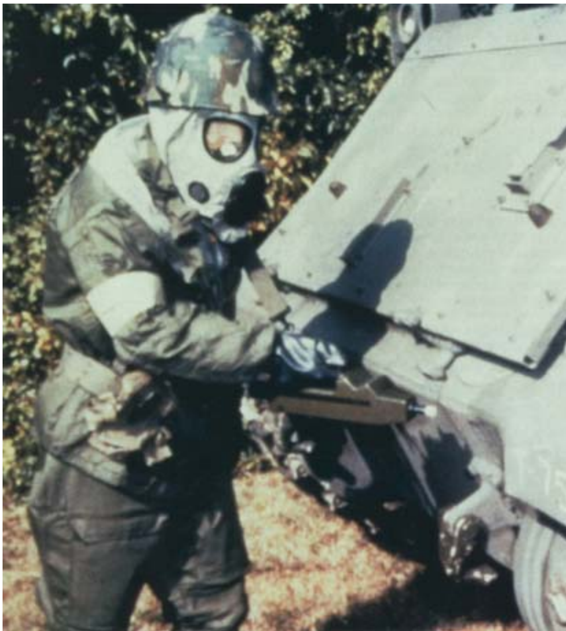
Fig. 6-14. Improved-Chemical Agent Monitor (I-CAM). The I-CAM detects vapors of chemical agents by sensing molecular ions of specific mobilities and uses timing and microprocessor techniques to reject common battlefield interferences. It consists of a drift tube, signal processor, molecular sieve, membrane, and expendable items such as batteries, confidence testers, and dust filters.
