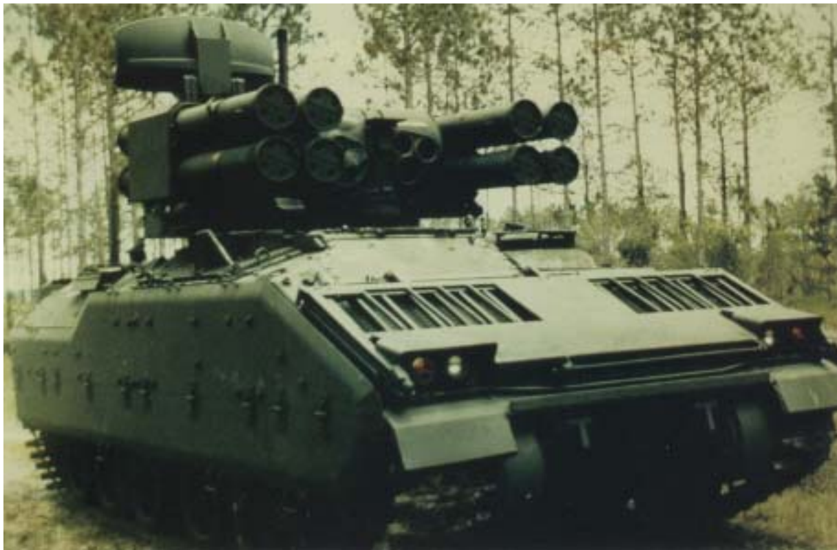
Fig. 6-13. Air Defense Antitank System. The ADATS is designed to operate autonomously or to use forward area air defense command, control, and intelligence data, during day or night, in obscurants, in adverse weather, and in battlefield environments where electronic and physical countermeasures are present. The system is operated by a crew of three: driver, gunner, and commander. This program was cancelled in the early 1990s both as a cost-saving measure and because the threat in Europe had changed.
