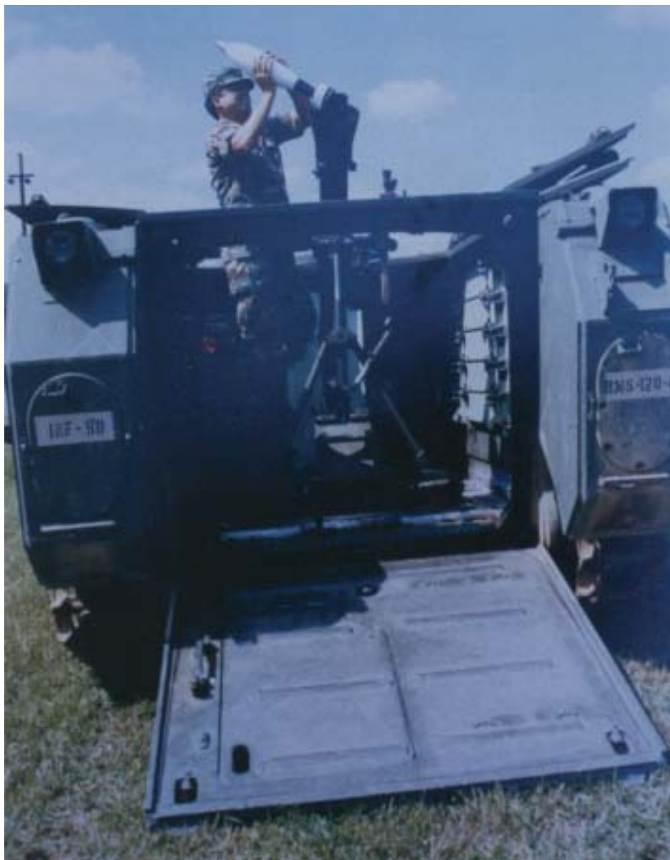
Fig. 6-7. 120-mm Battalion Mortar System (BMS-120). The BMS-120 provides dismounted (walking alongside) and mechanized infantry units increased range and lethality with high-explosive, illumination, and smoke-screening rounds. Concurrently with the acquisition of the BMS-120, a new family of enhanced ammunition is being developed. This M121 carrier-mounted configuration is shown with a BAD (blast attenuating device) mounted on the muzzle of the mortar.
