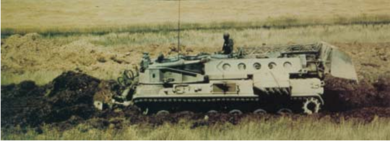
Fig. 6-20. Counterobstacle Vehicle (COV). The prototype COV pictured here is a highly mobile vehicle capable of clearing and creating major obstacles and emplacements. It is equipped with a combination bulldozer / mineplow and two telescopic arms. The arms are normally used with buckets, but can also accept a hammer, auger, lifting hook, grapple, and other attachments. These attachments enable it to move earth, breach minefields, knock down obstacles, dig defilade positions for armored vehicles, and excavate antitank ditches.
