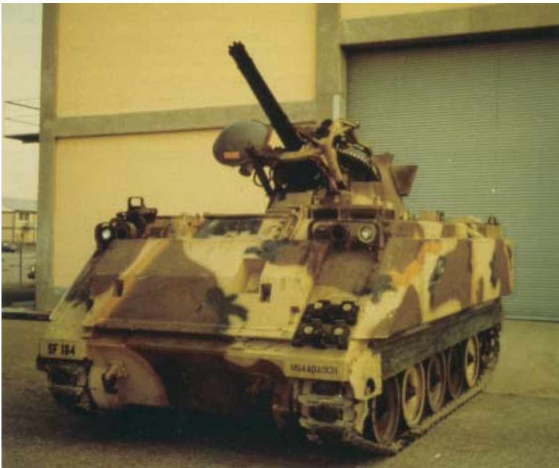
Fig. 6-18. M163A2 Self-Propelled 20-mm Vulcan Air Defense System (VADS). Major components of the M163A2 VADS include the M168 20-mm cannon, M61A1 director sight, AN/PVS-2 range-only radar, and the M741 chassis. It carries 1,000 ready 20-mm rounds in a linkless feed system.
