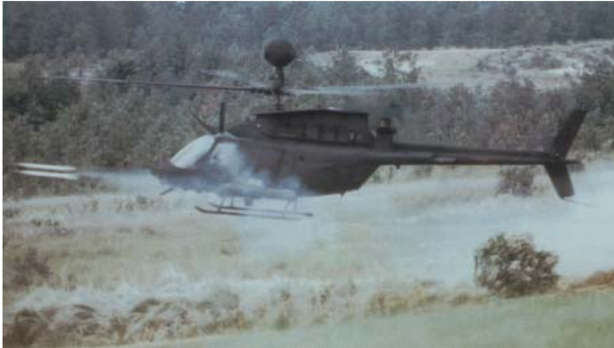
Fig. 6-16. Armed OH-58D Kiowa Warrior Scout Helicopter. The OH-58D uses a new drive train consisting of a four-bladed rotor, 650-hp engine and compatible transmission and tail rotor systems. Beginning in fiscal year 1991, the armed version was equipped with air-to-air Stinger missiles. An air-to-ground weapons suite will arm the aircraft with Hellfire missiles, Hydra 70 2.75-in. rockets, and / or a .50-caliber machine gun. The aircraft is operated by a crew of two, has a maximum gross weight of 5,500 pounds, and a maximum level speed of 118 knots.
