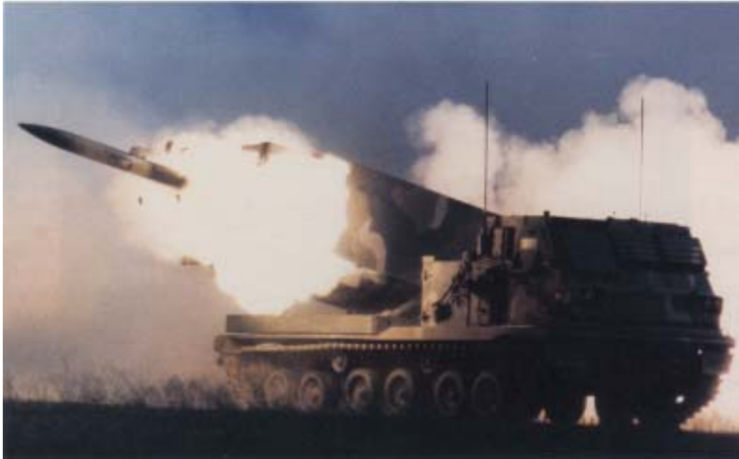
Fig. 6-2. The Multiple Launch Rocket System (MLRS). The MLRS is a free-flight artillery rocket system that improves the conventional, indirect-fire capability of the field army. It consists of a 12-round launcher mounted on a mobile, tracked vehicle. The MLRS is capable of launching rockets, with varying types of warheads, either one at a time or in rapid ripples, to ranges beyond 30 km.
