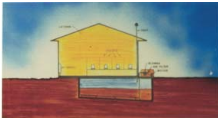
Fig. 6-9. Composting Toilet and Aerated Vault Toilet. Composting toilets, left, were developed in Sweden and have been used in the U.S. Army for many years. The breakdown of wastes is accomplished naturally by aerobic decomposition, without additional H 2 O or other chemicals. In the aerated vault toilet, right, waste is broken down into CO 2 and H 2 O by aerobic organisms. Aerobic decomposition occurs about 4-fold faster than anaerobic decomposition, thereby reducing pumping costs. Preventing anaerobic decay also greatly reduces the odors in the toilets.
