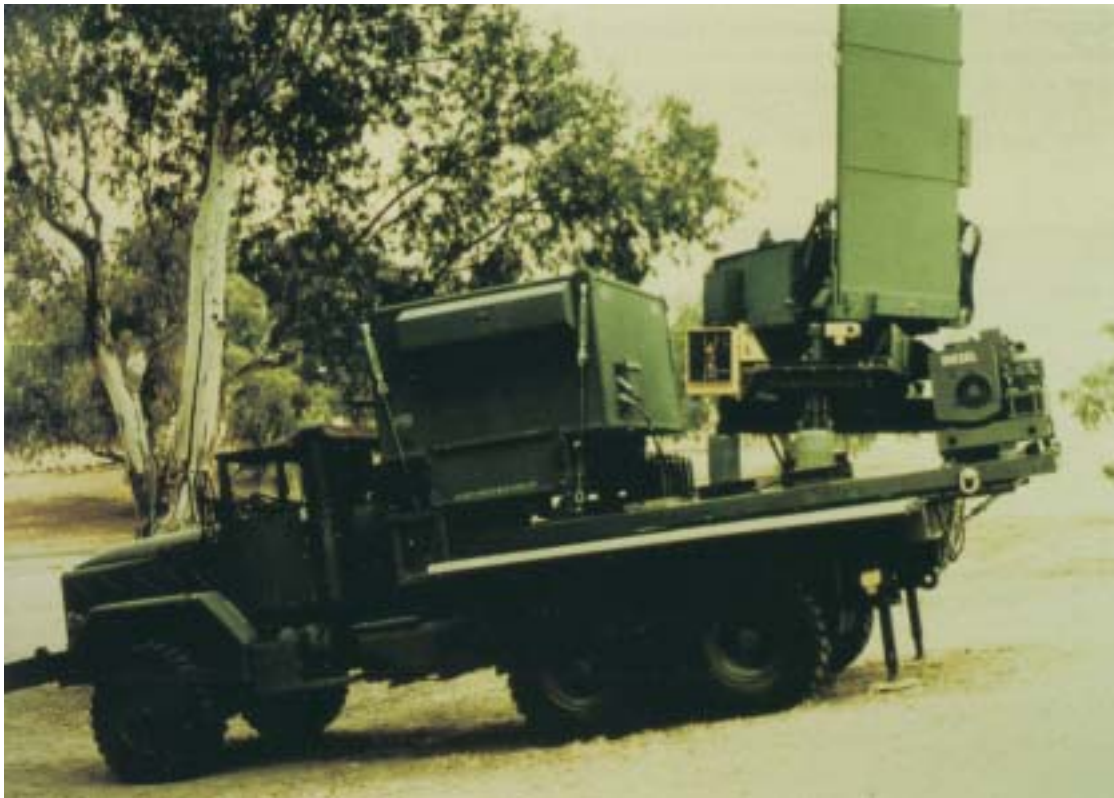
Fig. 6-15. Firefinder Mortar Locating Radar (MLR), Block II Program. The MLR is deployed close to the forward line of troops with direct support artillery battalions. In fiscal year 1990, the army approved the system's reconfiguration so it could be carried by 1¼-ton capacity HMMWVs (High-Mobility, Multipurpose, Wheeled Vehicle). Future improvements will also include eliminating the S-250 operations shelter, reduced emplacement time, faster access to data, increased program memory and digital map storage, improved throughput and processing, remote operation capability up to 100 m, and better probability of detecting the location of enemy weapons.
