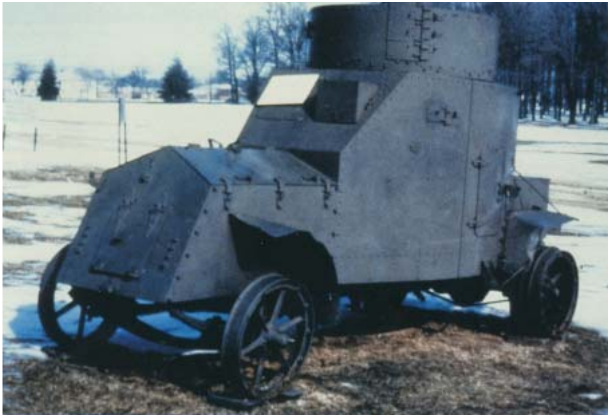
Fig. 6-5. White Armored Car (M1913-1914), shown at the U.S. Army Ordnance Museum, Aberdeen Proving Ground, Maryland. Built by the White Motor Company, this vehicle weighed about 2 tons and was a built-up armored truck. It had dual rear wheels with pneumatic tires and a caliber .30 Vickers-Maxim machine gun in the rounded turret. It was used by General Pershing's troops along the Mexican border in 1916 during their pursuit of Pancho Villa.
