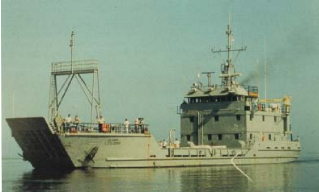
Fig. 6-11. Landing Craft Utility-2000 (LCU-2000). LCU-2000 ships are 174 ft long by 42 ft wide and displace 1,087 tons when fully loaded. Their speed is 12 knots and range is 5,000 miles. The main deck level houses the mess, sick bay, and recreation room. The crew quarters are on the second level; the pilot house is on top. A stern module contains the engine room and associated machinery.
