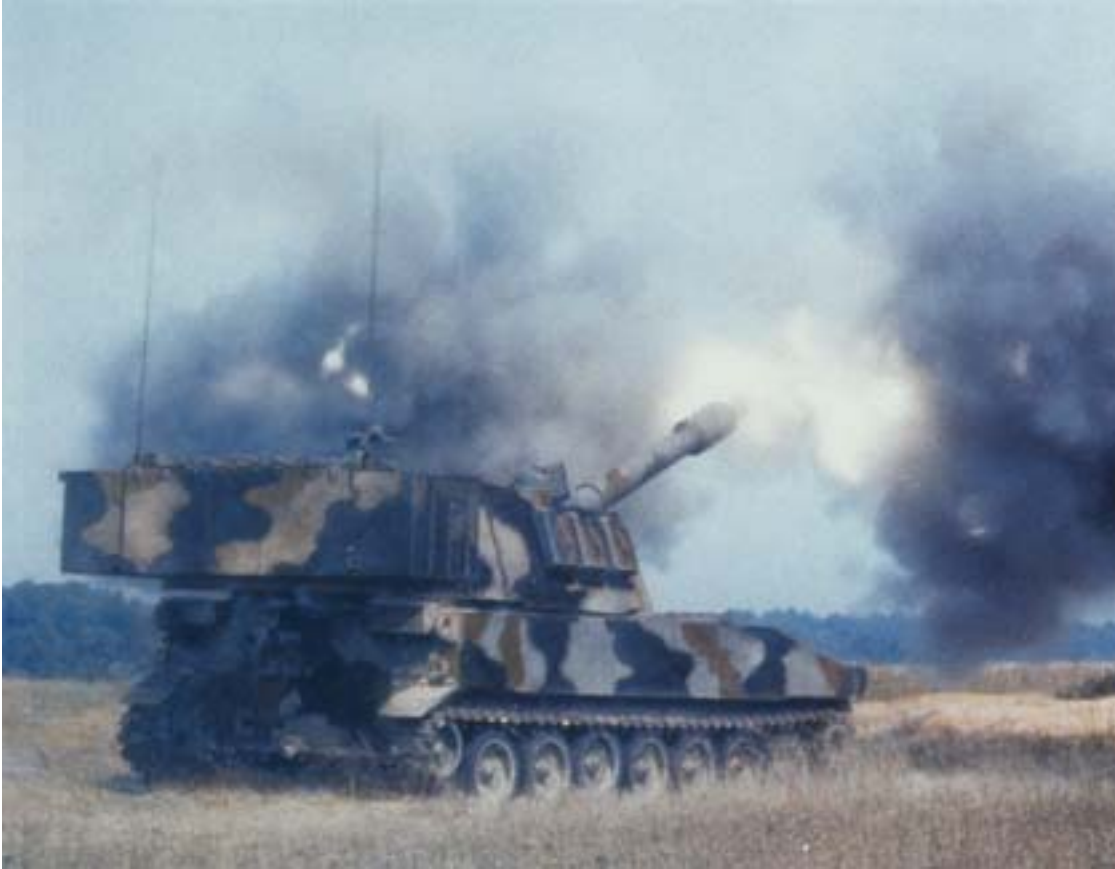
Fig. 6-8. The M109 155-mm Howitzer Improvement Program (HIP) Self-Propelled Howitzer (SPH). The HIP includes a new cannon and mount, an on-board fire-control system, a navigation system, automotive improvements, additional ballistic protection, NBC (nuclear-biological-chemical) protection for the crew, a driver's night-vision device, built-in test equipment, and secure communications. HIP modifications will be applied to all M109 SPHs not converted to M109A4 or M109A5, under the designation M109A6 Paladin, shown above.
