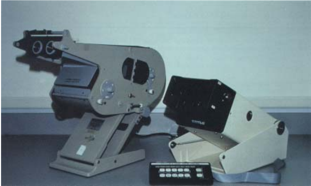
Fig. 8-1. The Armed Forces Vision Tester (AFVT), left, has been used for screening soldiers for decades and is still in use at most military entrance processing stations. The AFVT is mechanically operated, highly reliable, and is made of heavy-gauge steel. The AFVT is gradually being replaced by a new generation of lightweight, portable, and electronically operated vision screeners, such as the Titmus II Vision Screener, right. Other similar new vision screeners include the Optec 2000, manufactured by Stereo Optical, Inc., and the Sight Screener II, manufactured by American Optical Company.
