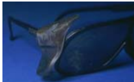
Fig. 23-2. (a) A short-range thermal blast induced significant damage to the face of this individual. The periocular area was spared by the patient's protective eyewear. (b) The polycarbonate lenses have been significantly pitted by the heat and flying debris. The blast was of sufficient intensity that its heat melted the side shields.
