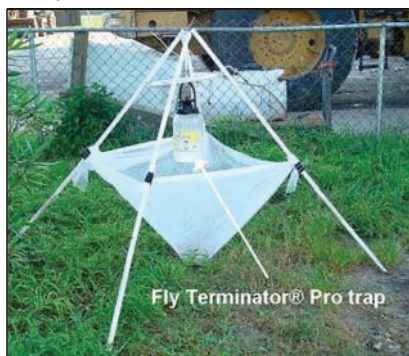
Figure 1. Fly trap and stand. Pyramid arrangement enabled use of the rain shield while keeping the trap at a useful height and minimizing ant contamination.
