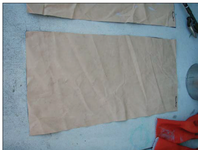
Figure 2. Vinyl tent strips (61 cm by 30.5 cm) used for residual insecticide efficacy studies against the sand fly Phlebotomus papatasi , a vector of cutaneous leishmaniasis in Afghanistan and the Middle East.
