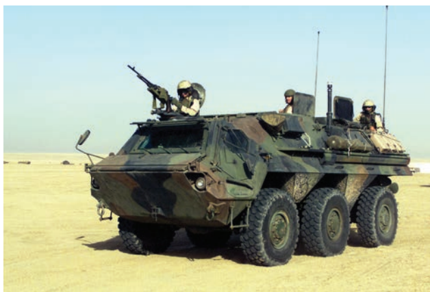
Figure 5-3. The M93 “Fox” nuclear, biological, and chemical reconnaissance vehicle.
