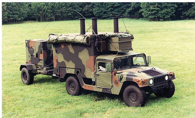
Figure 5-1. The Biological Integrated Detection System (BIDS) is a semi-automated biological agent detection/identification suite mounted on a dedicated heavy high mobility multipurpose wheeled vehicle. The system uses multicomplementary bio-detection technologies.
