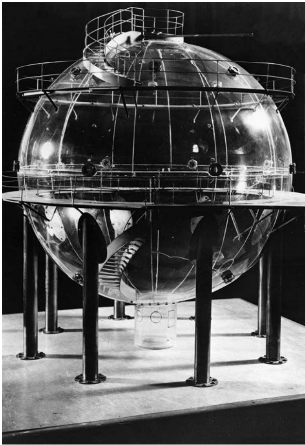
Figure 29-1. Design of the 1-million-liter sphere ball known as “Eight Ball,” which was used to expose the Operation Whitecoat volunteers to Francisella tularensis and C burnetii at Fort Detrick, Maryland.
