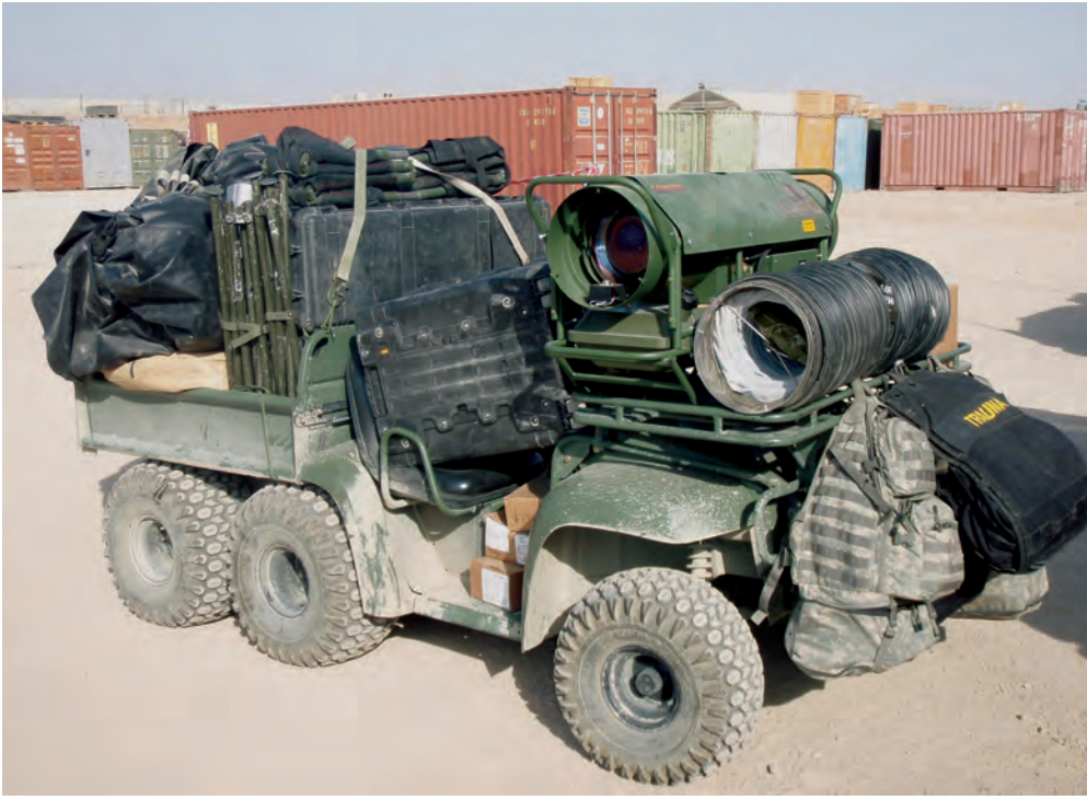
FIGURE 10-6. Early set-up (2007) of a non-doctrinal wheeled vehicle configured for forward surgical team (FST) missions in support of Special Operations forces. The vehicle would be transported via a rotary-wing aircraft to a far forward location. Photograph courtesy of LTC Kyle Remick, former commander of the 772nd FST.
