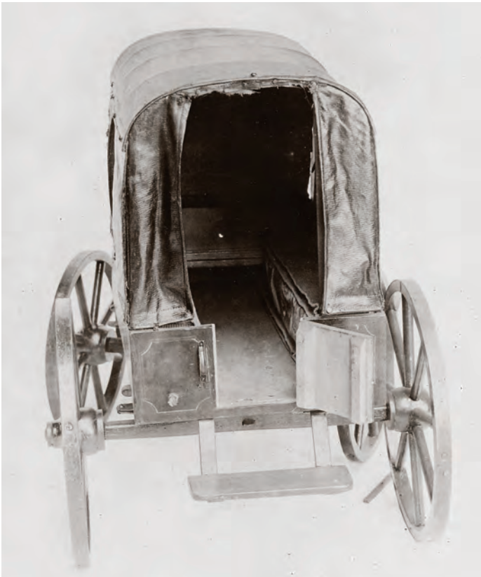
FIGURE 3-4. Views of the Letterman ambulance. The ambulance formed the centerpiece of the Ambulance Corps organized by Jonathan Letterman. The ambulances featured springs in their suspension that were much more comfortable for the occupants than a regular wagon. They were drawn by horse or mule with canvas roofs and sides of canvas. Two-wheel ambulances were followed by the four-wheel ambulance pictured here. Photograph courtesy of the National Library of Medicine, Image #19999137-2.
