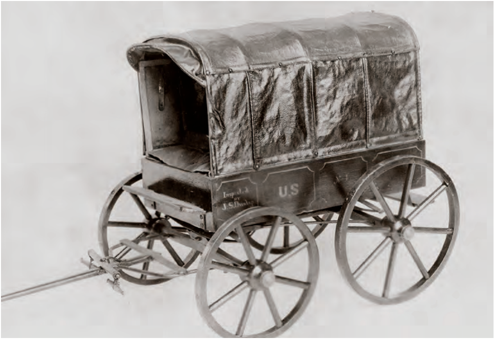
FIGURE 3-4. Views of the Letterman ambulance. The ambulance formed the centerpiece of the Ambulance Corps organized by Jonathan Letterman. The ambulances featured springs in their suspension that were much more comfortable for the occupants than a regular wagon. They were drawn by horse or mule with canvas roofs and sides of canvas. Two-wheel ambulances were followed by the four-wheel ambulance pictured here. Photograph courtesy of the National Library of Medicine, Image #19999137-2.
