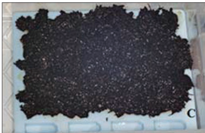
Figure 4. The embedding mold filled with RMGI restoration material covered with the smokeless tobacco/salivary substitute mix. The other 2 embedding molds were covered in a similar manner.
