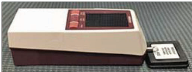
Figure 5. Surface roughness tester (Surftest SJ-210 profilometer).
