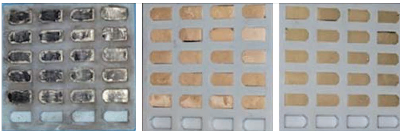
Figure 2. Amalgam (left), composite resin (center), and glass ionomer (right) restoration materials in embedding molds.
