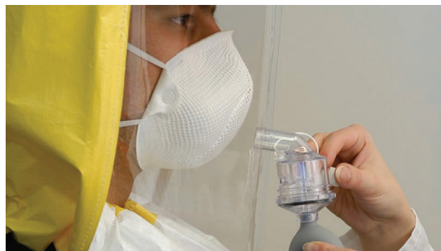
Figure 13-9. Qualitative fit testing is done by releasing a chemical with a recognizable odor into the hood space surrounding the respirator and determining whether the odor is detectable in the respirator's facepiece. Photograph courtesy of Brandon Gardner, Major, Medical Corps, US Army; US Army Medical Department Center and School, Fort Sam Houston, TX.
