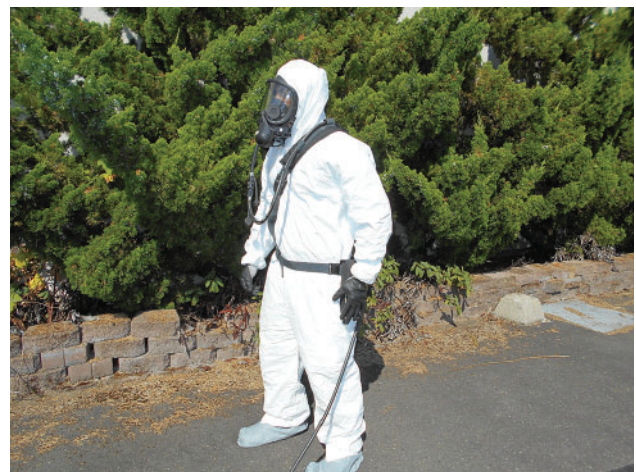
Figure 13-5. The full-face air-line respirator provides the wearer breathing air in hazardous environments. The respirator can be worn for a full work shift.
