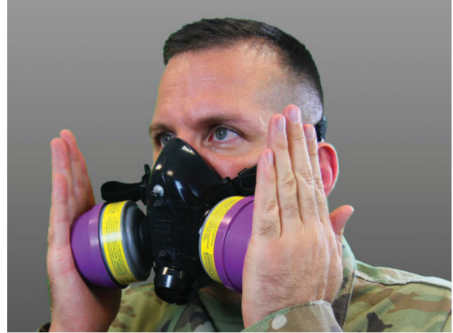
Figure 13-11. A negative seal check is a function check of the respirator performed by the wearer who inhales forcefully while covering the intake ports of the respirator. Photograph courtesy of Brandon Gardner, Major, Medical Corps, US Army; US Army Medical Department Center and School, Fort Sam Houston, TX.
