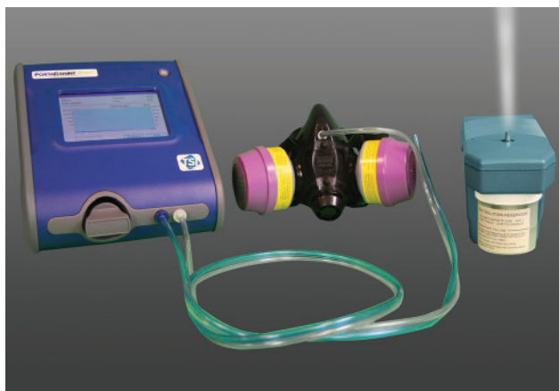
Figure 13-8. Quantitative fit testing will measure the concentration of particulates outside the mask and compare it with the concentration inside the mask to assure mask seal quality. Photograph courtesy of Brandon Gardner, Major, Medical Corps, US Army; US Army Medical Department Center and School, Fort Sam Houston, TX.
