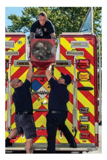
**Figure 15-10.** Lowering of a smoke ejector fan before ergonomic intervention. Notice the firefighters' poor postures and force requirements as they reach to move the fan. Photograph courtesy of Christina Graber, US Army Public Health Center, Aberdeen Proving Ground, MD. Used with
