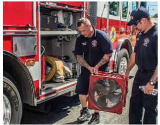
**Figure 15-11.** Firefighters relocate a smoke ejector fan after an ergonomic intervention. Notice how relocating the fan from the top of the fire truck to the rear bumper allows for easier access.
