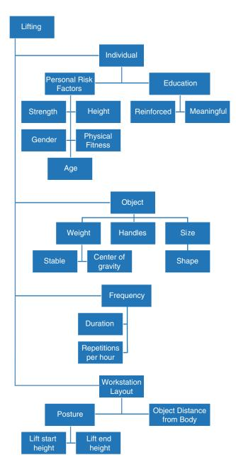
**Figure 15-7.** There are multiple risk factors to consider when a lift takes place to ensure a worker will benefit from ergonomic interventions.
