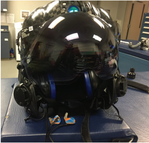
Figure 16-3. Aircrew helmet with communicating ear plugs. Photograph courtesy of Christianne N. Opresko, Major, Medical Corps, US Air Force; Eglin Air Force Base, FL.
