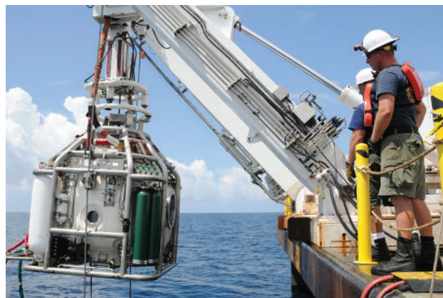
Figure 17-13. The dive bell component of the Flyaway Saturation Diving System, which is used to transport saturation divers to and from a large compression chamber on the surface and the ocean depths where they perform their work. Gulf of Mexico, May 9, 2012 - Navy Diver 1st Class Alvin Carter, right, a reserve component sailor certified to mix gases for breathing in deep-water diving, watches as a winch hoists a manned dive bell from a depth of more than 600 feet, more than 65 miles south of the coast of Panama City Beach, FL. US Navy photo by Mass Communication Specialist 2nd Class Charles E. White (Released). Reproduced from: http://www.navy.mil/view_image.asp?id=123795/ .
