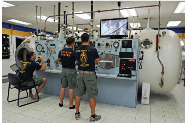
Figure 17-14. Double-lock hyperbaric chamber. Santa Rita, Guam, February 25, 2015 - US Naval divers monitor a patient during a demonstration for patient care due to decompression illness in the hyperbaric chamber. US Naval Base Guam is home to the only recompression chamber in the region and provides treatment to military and civilian personnel from Guam and the Micronesia Islands. US Navy photo by Mass Communication Specialist 2nd Class Chelsy Alamina (Released). Reproduced from: http://www.navy.mil/view_image.asp?id=192715 .
