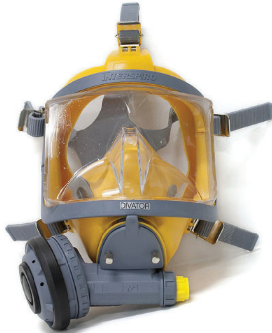
Figure 17-4. The US Navy Mk 20 Mod 0 surface-supplied, open-circuit, lightweight system with full facemask is limited to a depth of 60 fsw (18 msw) for applications such as diving in mud tanks and enclosed spaces.
