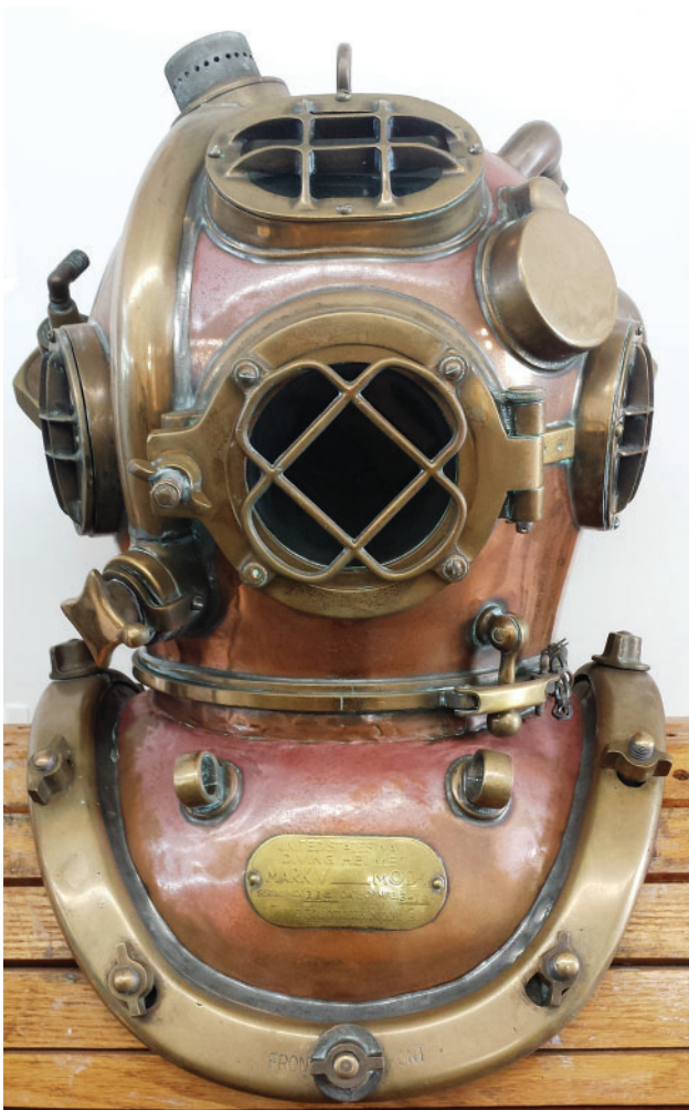
Figure 17-3. The US Navy Mk V Mod 1 diving helmet.
