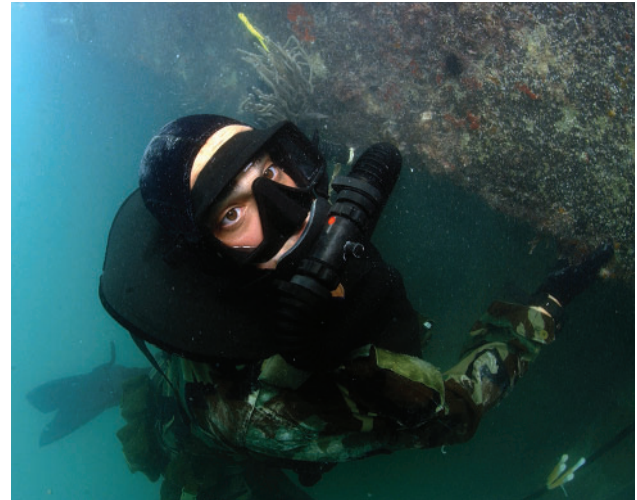
Figure 17-6. The Mk 25 Underwater Breathing Apparatus. May 18, 2006 - A US Navy SEAL (Sea, Air, Land) hangs on to a pier during a Combat Swimmer Training dive. US Navy photo by Senior Chief Mass Communication Specialist Andrew McKaskle (Released). Reproduced from: http://www.navy.mil/view_image.asp?id=37909 .
