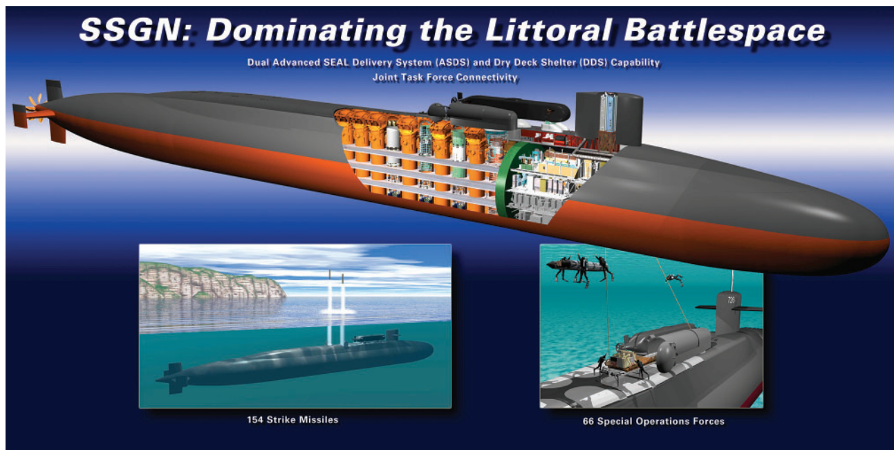
Figure 19-4. The guided missile submarine can support and launch up to 154 Tomahawk missiles, a significant increase in capacity compared to other platforms. The 22 missile tubes can also carry other payloads, such as unmanned underwater vehicles, unmanned aerial vehicles, and Special Forces equipment. This new platform can carry and support more than 66 Navy sea, air, and land unit personnel and insert them clandestinely into potential conflict areas. Reproduced from US Navy news photo 030814-N-0000X-006.
