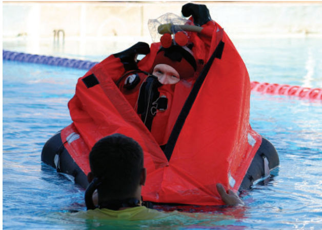
Figure 19-8. A sailor assigned to the Los Angeles-class nuclear-powered attack submarine, USS Key West (SSN-722), receives training with the MK 10 submarine escape immersion equipment suit. Reproduced from US Navy news photo 041012-N-0879R-007.
