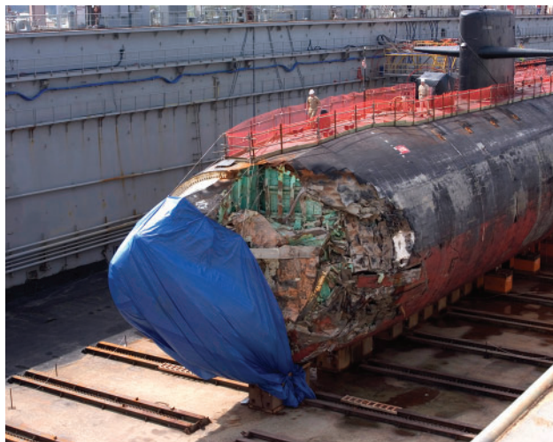
Figure 19-5. The Los Angeles-class nuclear powered fast-attack submarine, USS San Francisco (SSN-711), is pictured in dry dock undergoing damage assessment after a high-speed collision with an underwater seamount. Reproduced from US Navy news photo 050127-N-4658L-030.
