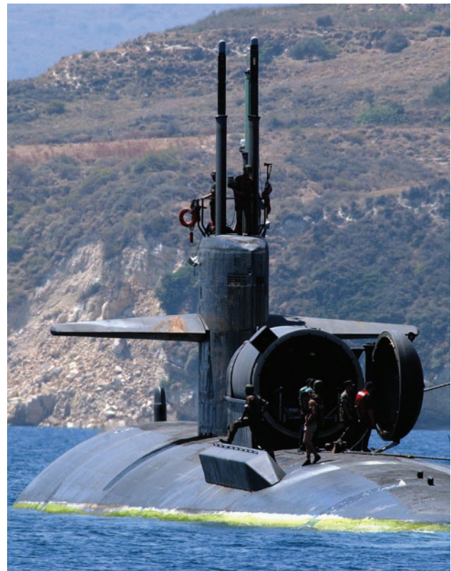
Figure 19-3. The Los Angeles-class nuclear-powered attack submarine, USS Dallas (SSN-700), with dry deck shelter. Reproduced from US Navy news photo 040719-N-0780F-070.
