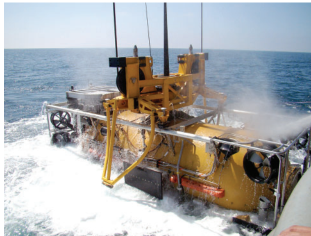
Figure 19-9. The pressurized rescue module is recovered from the water after performing a submarine rescue exercise with the Chilean submarine, CS Simpson , off the coast of San Diego, California, September 18, 2008. US Navy photo by Communication Specialist 2nd Class Alexia M. Riveracorrea. Reproduced from US Navy news photo 080918-N7029R-115.
