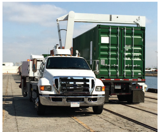
Figure 22-15. Cargo and vehicle inspection systems. The radiation beam is directed toward the detector tower mounted on the truck. This system can acquire both transmission and backscatter images. The x-ray source is located inside the truck box and the radiation beam is directed outward. Photographs courtesy of Leidos.
