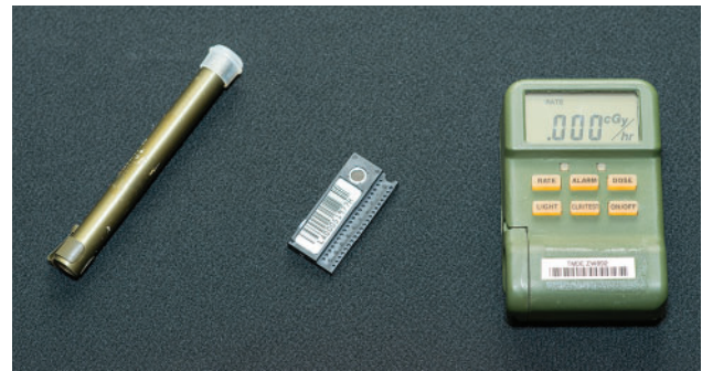
Figure 22-21. Three types of dosimeters. The instrument on the left is an IM 93A/UD pocket dosimeter used in a tactical military environment. The IM-93A/UD can detect gamma radiation between 0 and 600 R. The middle instrument is a thermoluminescent dosimeter (TLD) used in both medical and industrial settings within the Department of Defense to determine radiation doses workers are exposed to. TLDs also have been used in tactical environments. The four tissue-equivalent materials within a TLD can show the radiation dose from different forms of radiation. The range of the TLD is from 0.5 mSv to 10 Sv. On the right is the AN/UDR-13 electronic dosimeter, which is used extensively in the military. The compact and rugged AN/UDR-13 is capable of detecting gamma and neutron radiation doses, as well as the dose rate for gamma radiation. This dosimeter's capability is 1 to 999 cGy for dose detection, and 0.1 to 999 cGy/h for dose rate. Photograph courtesy of the US Army Public Health Command, Aberdeen Proving Ground, Maryland.
