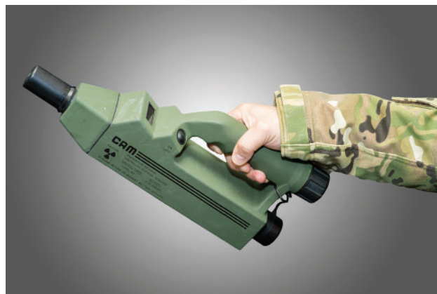
Figure 22-13. The chemical agent monitor (CAM) contains up to 15 mCi of nickel 63 used to ionize air molecules as the air passes through the CAM. The CAM is used to detect nerve and mustard chemical agents. Photograph courtesy of the US Army Public Health Center.
