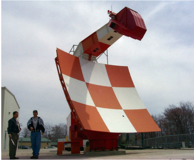
Figure 23-11. A microwave radar system installed at an Army depot. The waveguides feed the radio frequency power through the arm at the top of the antenna.
