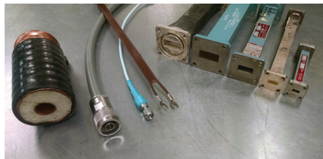
Figure 23-8. Assortment of conductor and waveguide transmission lines. The brown two-wire transmission line was salvaged from an old television set-top antenna. The light green cable handles the smallest amount of power transmission, while the coaxial cable section on the far left handles the most power. The waveguides increase in frequency from left to right.
