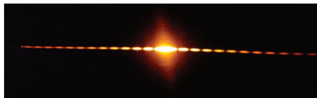
Figure 23-7. Single slit diffraction physics experiment showing the interference pattern of spatially coherent light.
