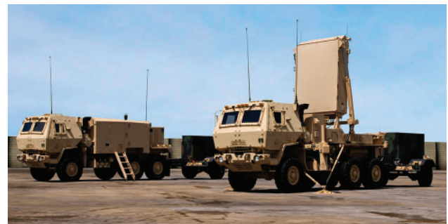
Figure 23-12. A trailer-mounted phased array radar system. Note that there is no defined parabola dish on the antenna. There is a red covering on the antenna for absorbing radio frequency radiation that attenuates the output power during maintenance or repair work; it is removed during operation.
