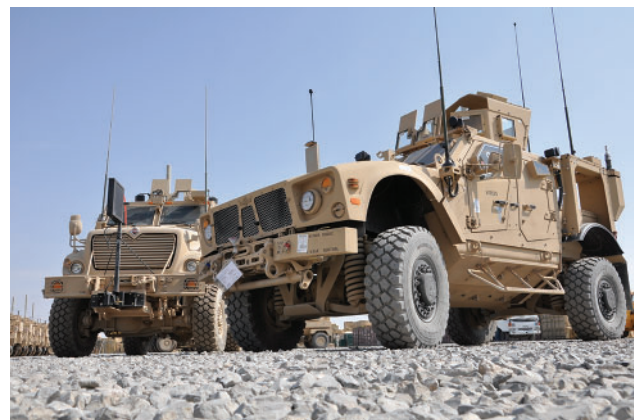
Figure 23-9. A mine-resistant, ambush-protected (MRAP) vehicle provides a variety of radio frequency communication systems. The most prevalent are the omnidirectional very high frequency (VHF) and ultra-high frequency (UHF) antennas. US Army photo by Specialist Elisebet Freeburg, Joint Sustainment Command–Afghanistan, PAO. Reproduced from: https://www.army.mil/e2-images/2009/10/23/53959/index.html
