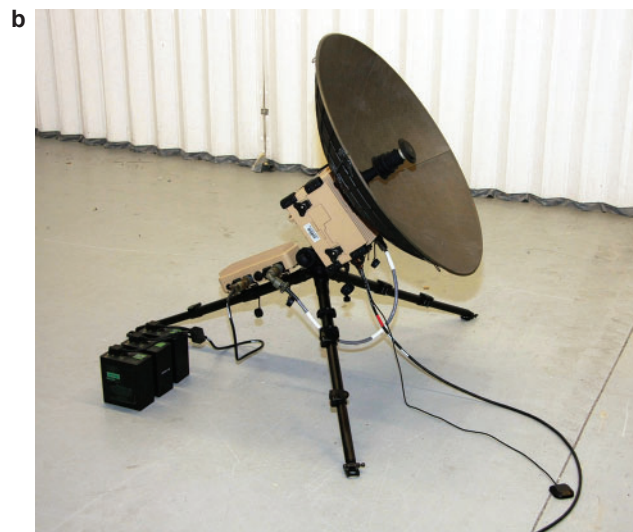
Figure 23-10. Two common very small aperture terminal (VSAT) deployments for portable operations: (a) a trailer-mounted AN/TSC-208; (b) a part of the AN/TSC-203 Global Response Intelligence Terminal.
