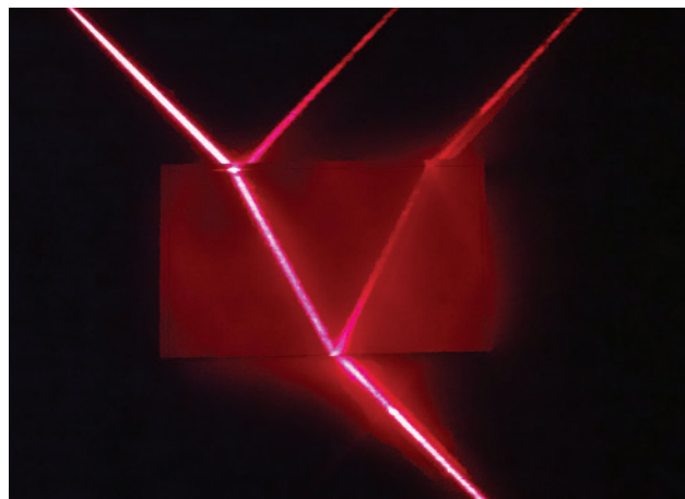
Figure 23-5. Refraction of laser light through a clear acrylic block. Although the acrylic is clear, a slight specular reflection occurs at each of the surfaces where the refraction occurs.
