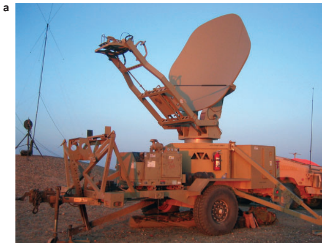
Figure 23-10. Two common very small aperture terminal (VSAT) deployments for portable operations: (a) a trailer-mounted AN/TSC-208; (b) a part of the AN/TSC-203 Global Response Intelligence Terminal.
