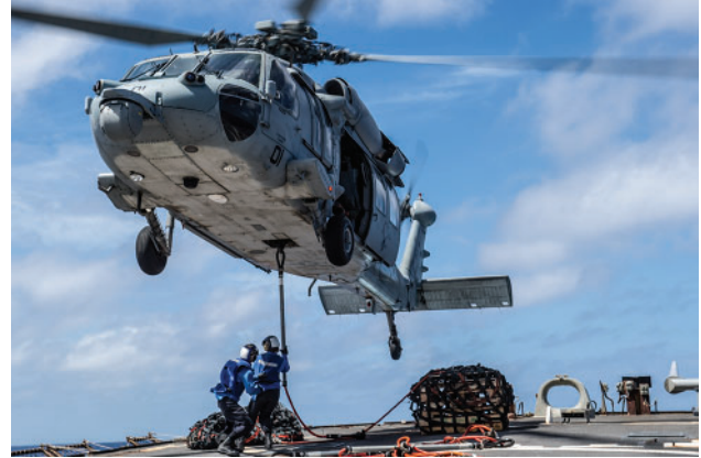
Figure 26-2. Two seaman attach cargo pendants to an MH-60S Sea Hawk helicopter, assigned to Helicopter Sea Combat Squadron 25 (HSC-25), on the flight deck of guided-missile destroyer USS Barry (DDG 52).
