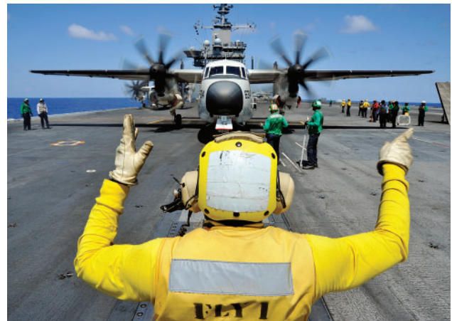
Figure 26-4. An aviation boatswain’s mate directs a C-2A Greyhound high-wing cargo aircraft assigned to Carrier Airborne Early Warning Squadron 120 (VAW-120) onto a catapult as it prepares for takeoff on flight deck of the aircraft carrier USS Harry S. Truman (CVN 75).
