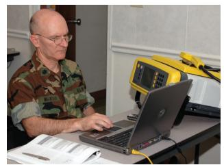
**Figure 3-7**. Commander Richard Maiello, an industrial hygienist attached to the Forward Deployed Preventive Medicine Unit Seven (FDPMU-7), conducts training on the Chemical Volatile Organic Compound Unit, which is used to screen soil, water, and air for the detection of toxic materials such as chemical, biological, and radiological agents. US Navy photo by Photographer's Mate 2nd Class Steven P. Smith. Reproduced from: http://www.navy.mil/view\_image.asp?id=36275
